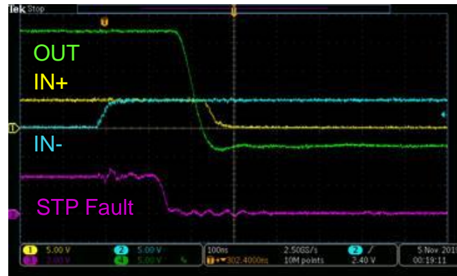
Shoot-through prevented and STP Fault triggered
