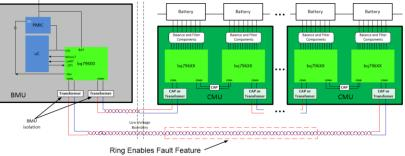
• We've designed a custom TI proprietary protocol specifically to interface with the BQ7961X family. A demo board and software have been designed to provide example solutions.
