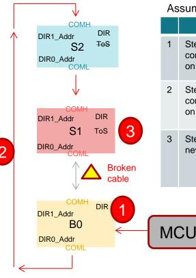
Procedure for MCU to set up reverse communication in daisy chain (south to north)
