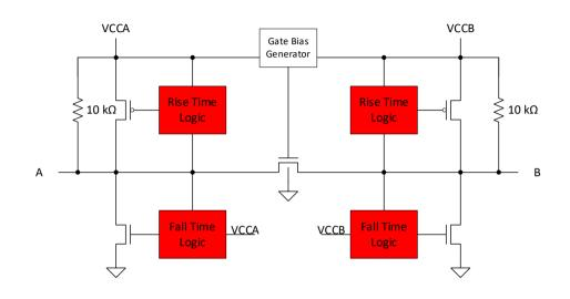
**Example of Rise Time & Fall Time Accelerator Circuit**
