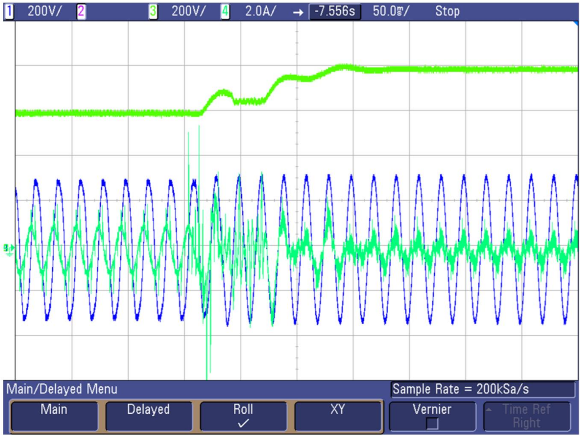
TIDA-01606, Vbus 800 V, Vac 230 startup waveform
