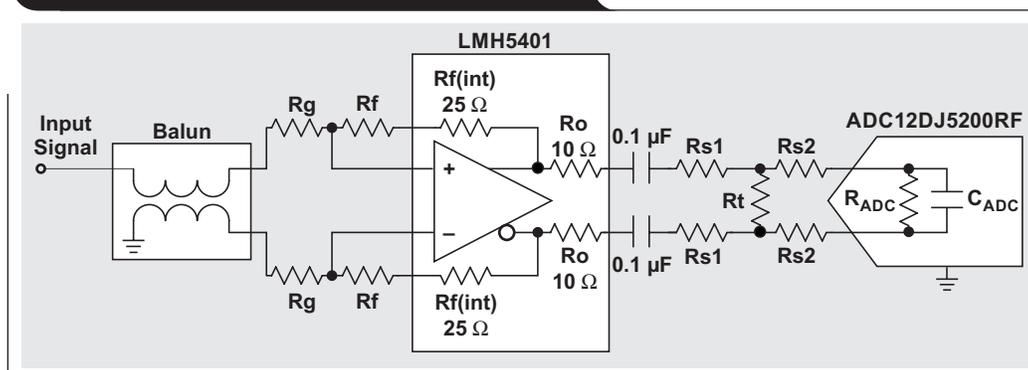
For example, a simple 50- $\Omega$  resistor with a 5% tolerance, 1,000 ppm/ $^{\circ}\text{C}$  over a  $-40^{\circ}\text{C}$  to  $+85^{\circ}\text{C}$  temperature range (125 $^{\circ}$ ) and a life drift of 2% over 1,000 hours would yield a resistance error of  $\pm 9.75 \Omega$ .
