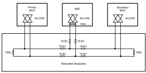
Figure 8-2. MicroTCA Redundant Clock Distribution Interface Example
