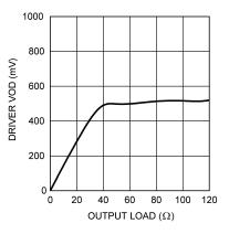
Figure 5-1. DS91D176 Driver Output Amplitude as a Function of Output DC Load
