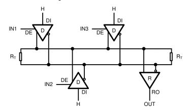
Figure 11-1. Wired-OR Circuit with Three M-LVDS Drivers and One Type 2 Receiver
