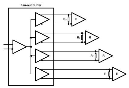
Figure 10-1. Signal Distribution with Point-to-Point Links
