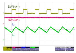
Figure 41. 36-V Buck Region With 40-A Load—Inductor Current Waveforms
