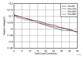
Figure 9. Load Regulation of Parallel Power
