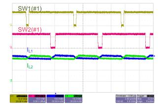
Figure 43. 12-V Buck-Boost Region With 40-A Load—Inductor Current Waveforms
