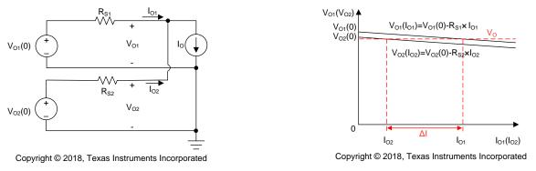
Figure 2. Equivalent Model
