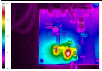
Figure 34. 40-A Load Thermal Condition in 36-V Buck Region—First Board
