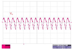
Figure 51. Output Voltage Ripple in 9-V Boost Region—40-A Load
