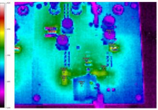
Figure 37. 40-A Load Thermal Condition in 12-V Buck-Boost Region—Second Board
