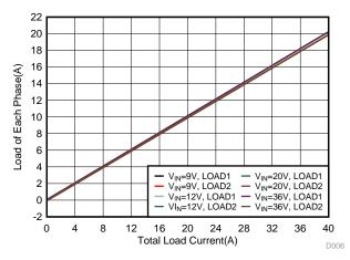
Figure 6. Load Distribution of Two Phases(Interleaved)
