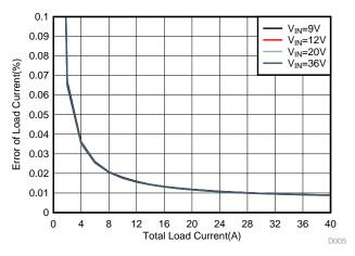
Figure 5. Error of Load Current(Interleaved)
