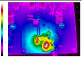
Figure 35. 40-A Load Thermal Condition in 36-V Buck Region—Second Board
