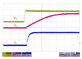
Figure 32. 40-A Start-Up in 9-V Boost Region—Total Output Current Waveform
