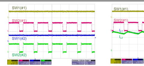
Figure 44. 9-V Boost Region With 40-A Load—Four Switch Nodes
