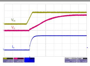
Figure 28. 40-A Start-Up in 36-V Buck Region—Total Output Current Waveform
