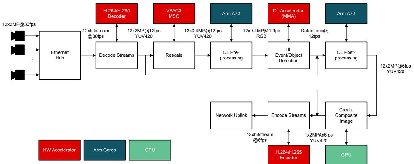
**Figure 3-1. AI Box Block Diagram With Data Flow on AM69A**
