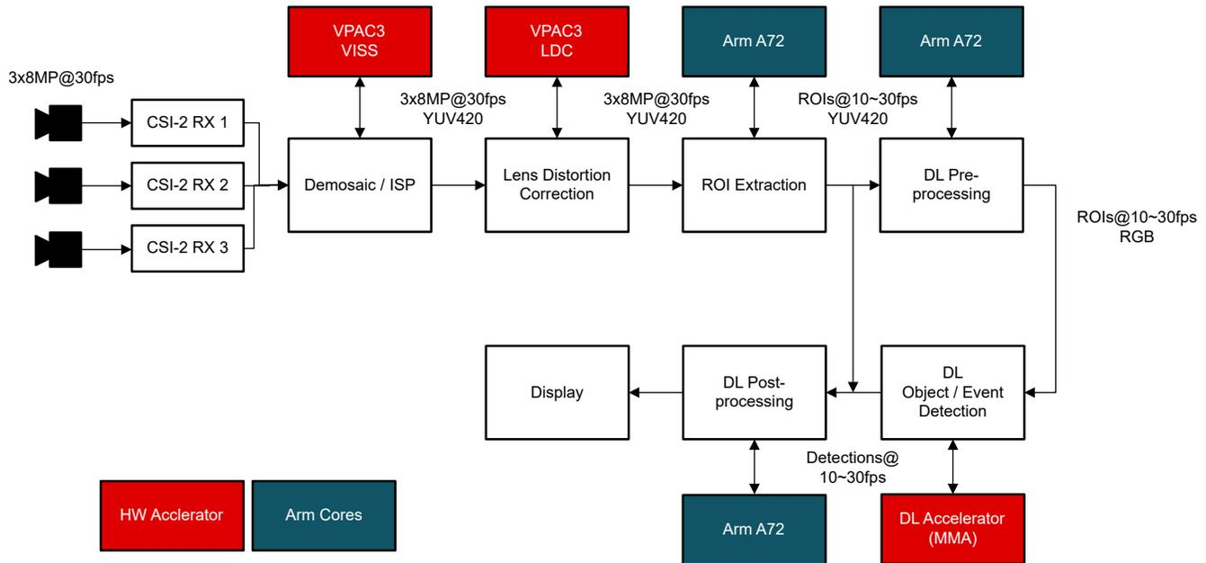
**Figure 3-2. Machine Vision Block Diagram With Data Flow on AM69A**
