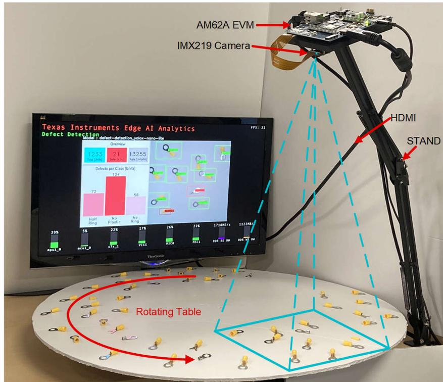
**Figure 4-2. Defect Detection Demo Setup (Only part of the rotating table is within camera frame to emulate a conveyor belt.)**
