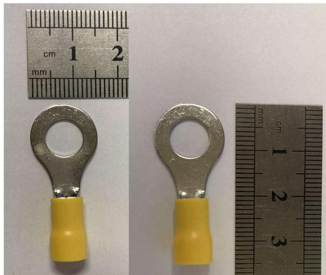
**Figure 2-1. Tests Samples Used for the Defect Detection Demo, Ring Crimp Terminals Connectors**
