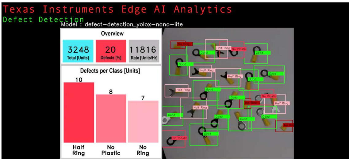
**Figure 1-1. Screenshot of the Defect Detection End Application Using AM62A (Right side is a live video feed with color boxes marking the detected objects. Left side is a graphical quality control dashboard.)**
