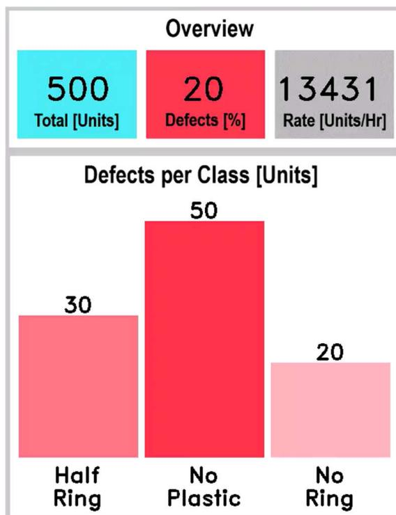
**Figure 5-1. Dashboard Results of the Accuracy Experiment With 50 Samples and 10 Repeated Tests (the defect detection application achieved 100 % accuracy)**
