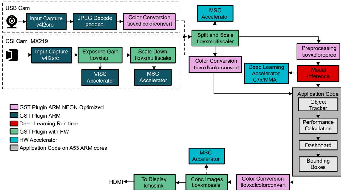
**Figure 4-1. Full System Flow Including Application Code and gstreamer Pipeline With Two input Options: a USB camera or a CSI IMX219 camera. The defect detection application supports the two input options.**
