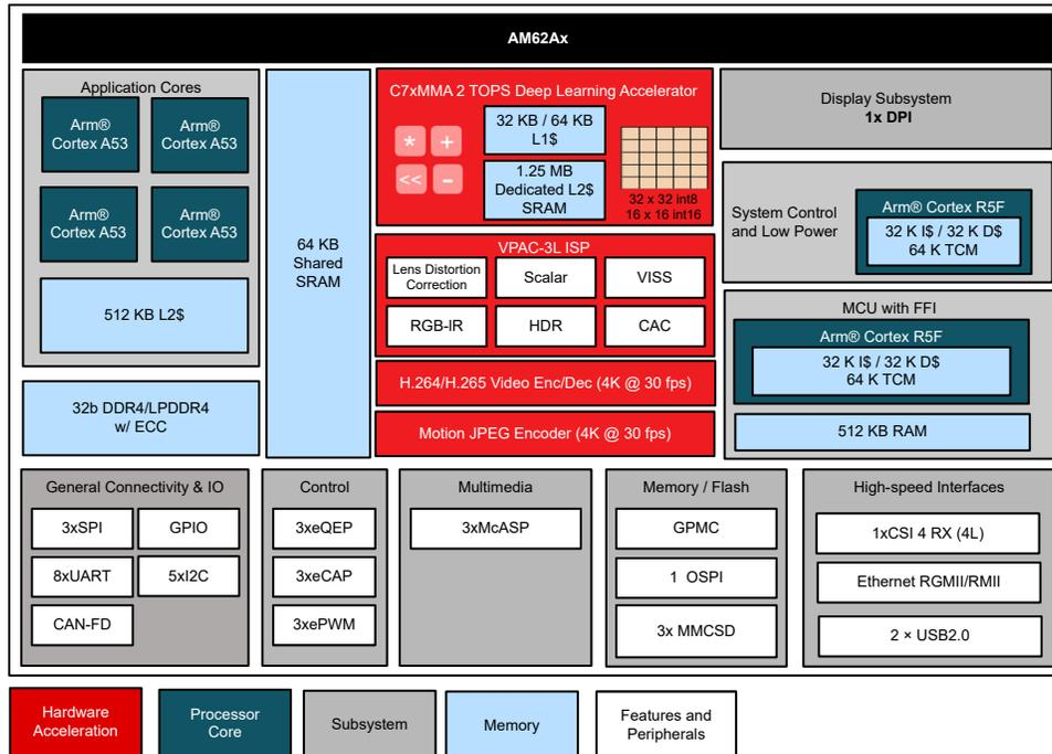
**Figure 1-2. AN62Ax Simplified Block Diagram**
