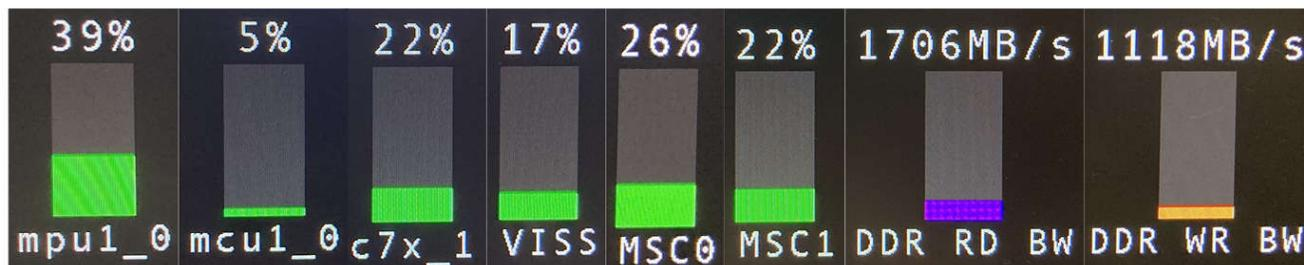
**Figure 5-2. Core Load Graph Bar Shown at the Bottom of the Defect Detection Demo Using tiperfoverlay gstreamer Plugin (the figure is edited to appropriately fit in the page)**
