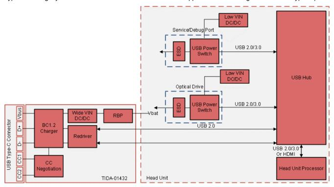
Figure 1. Passive Media Hub System Block Diagram
