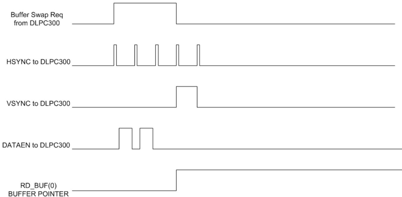
**Figure 7. Buffer Swap Timing for Stored Pattern Mode**
