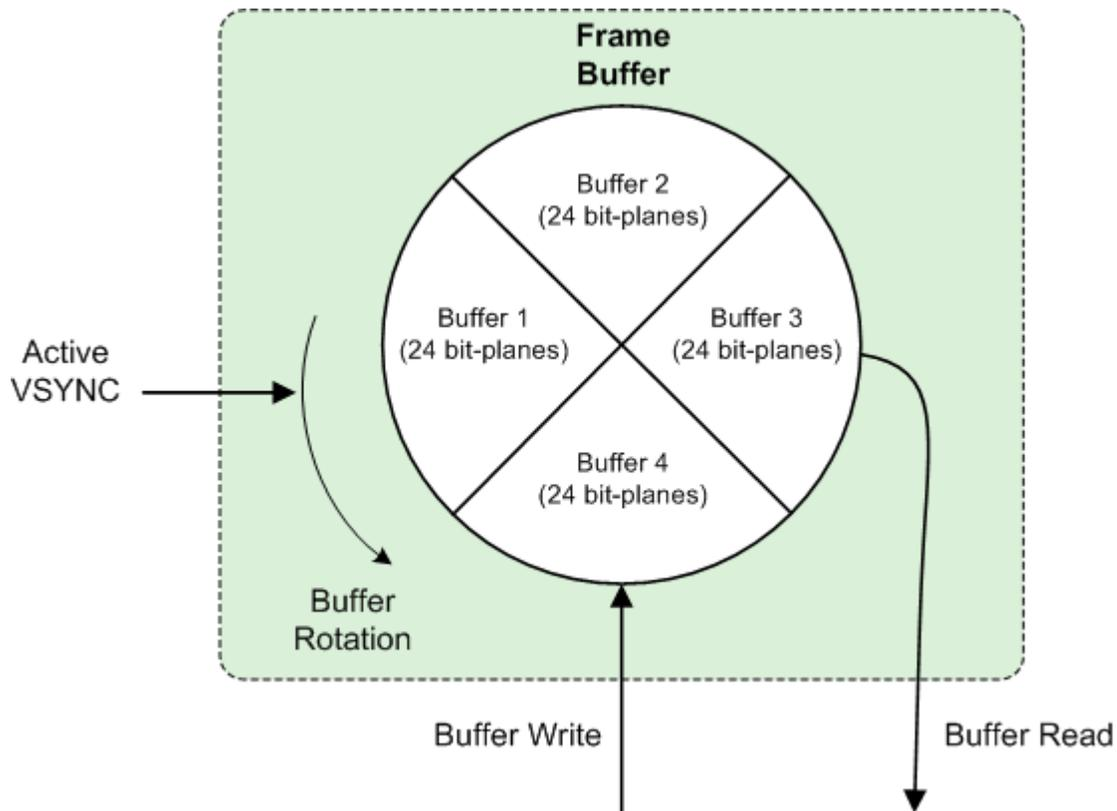
**Figure 4. Frame Buffer During Real-Time Streaming Video Mode**
