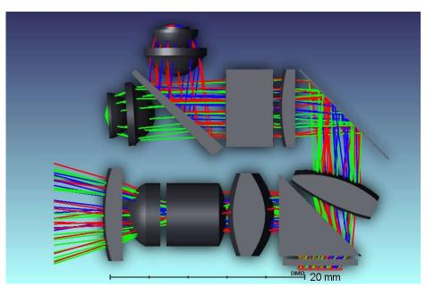
Figure 4-5. .2 WVGA (DLP2010) Optical Module Example
