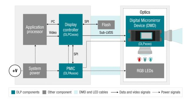
Figure 4-1. Typical DLP Display Block Diagram
