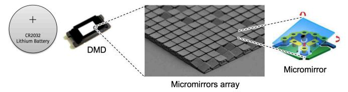
Figure 3-1. Digital Micromirror Device
