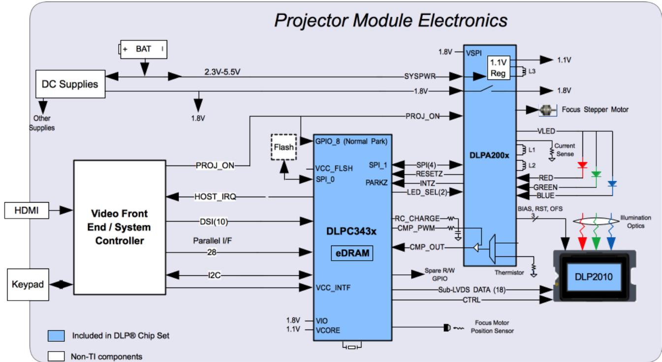
Figure 11. Typical DLP AM-HUD System Block Diagram
