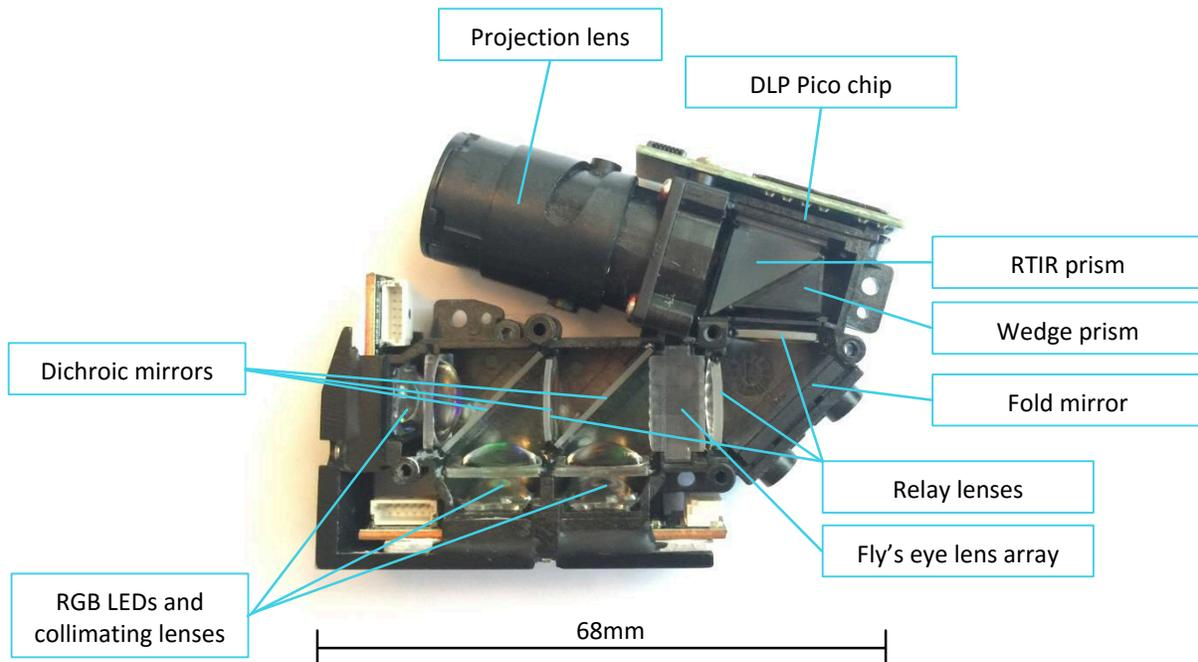
**Figure 1-2. Optical Components in an Example Pico Projection Optical Module Dimensions: 68×57×15 mm<sup>3</sup>**
