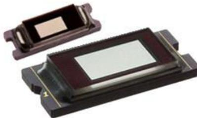
**Figure 3-2. A 0.2" Diagonal DMD (e.g. DLP2010) Compared to a 0.45" Diagonal DMD (e.g. DLP4501)**
