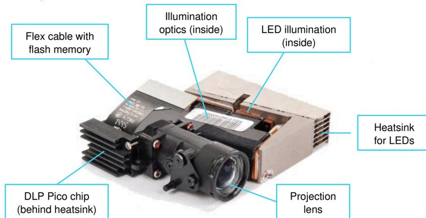
**Figure 1-1. Example DLP2010 Projection Optical Module - Dimensions: 44 × 48 × 14 mm<sup>3</sup>**
