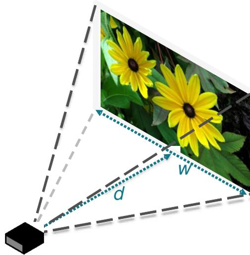
$$\text{Throw ratio} = \frac{(d)\text{distance from projection lens to the image}}{(w)\text{horizontal width of the image}}$$
