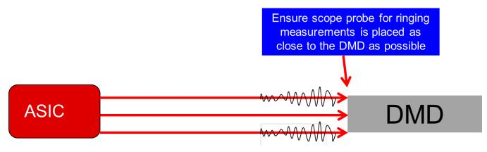
Figure 8. Measurement of DMD Signal Quality
