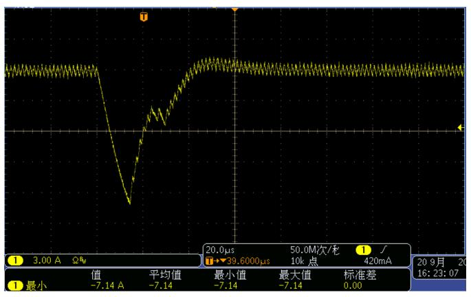
Figure 17. Reverse Current at VIN = 19 V, Inductor at 4.7 µF, and Output Capacitor at 44 µF
