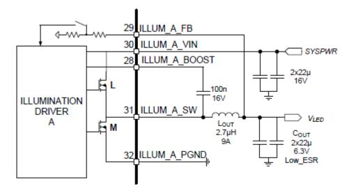
Figure 14. DLPA3000 Illumination Driver Circuits
