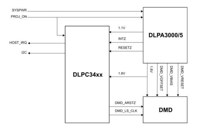
Figure 4. Critical Signals in DLPC34xx System
