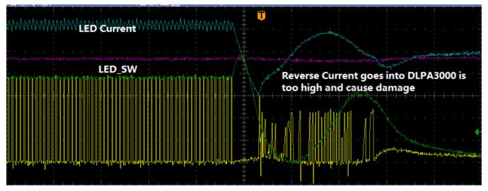
Figure 15. High Reverse Current Could Damage the Part
