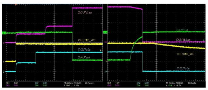
Figure 11. DMD Power On and Power Off Sequence
