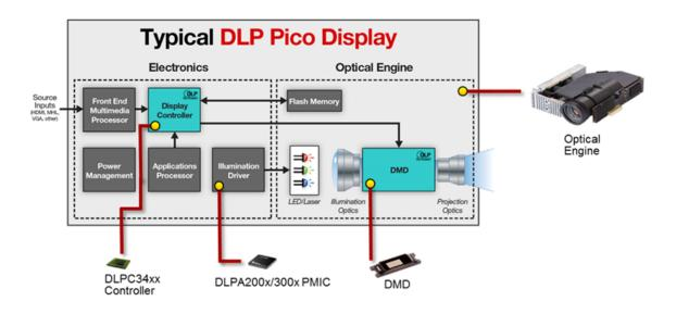
Figure 1. Typical DLP™ Pico System Block Diagram
