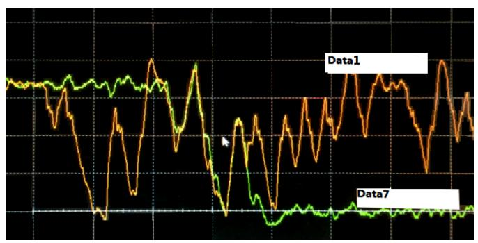
Figure 10. Data Signal Integrity Issues – Reflections, Discontinuities, and Noise
