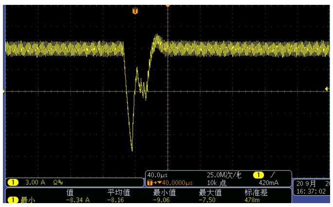
Figure 16. Reverse Current at VIN = 19 V, Inductor at 2.7  $\mu$ H, and Output Capacitor at 44  $\mu$ F
