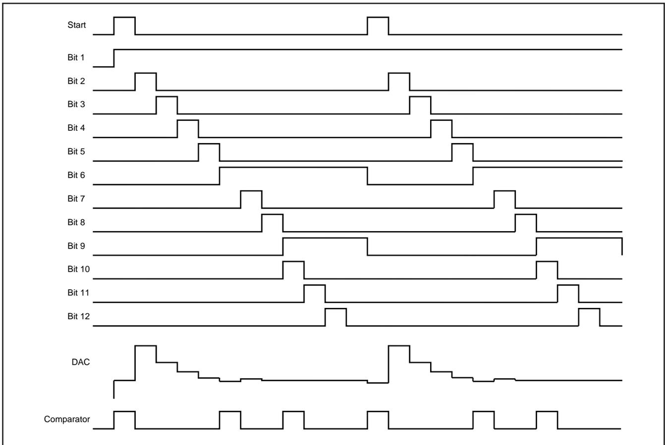
FIGURE 78. Timing Diagram of a Successive Approximation Converter.
