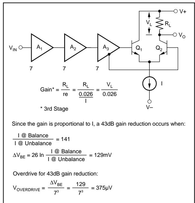
FIGURE 21. Gain Reduction to Stop Comparator Oscillation.
