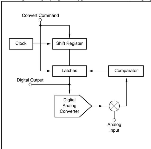
FIGURE 76. Block Diagram of Successive Approximation Analog-to-Digital Converter.
