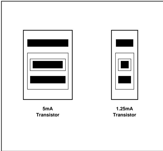
FIGURE 59. Scaled Transistors.
