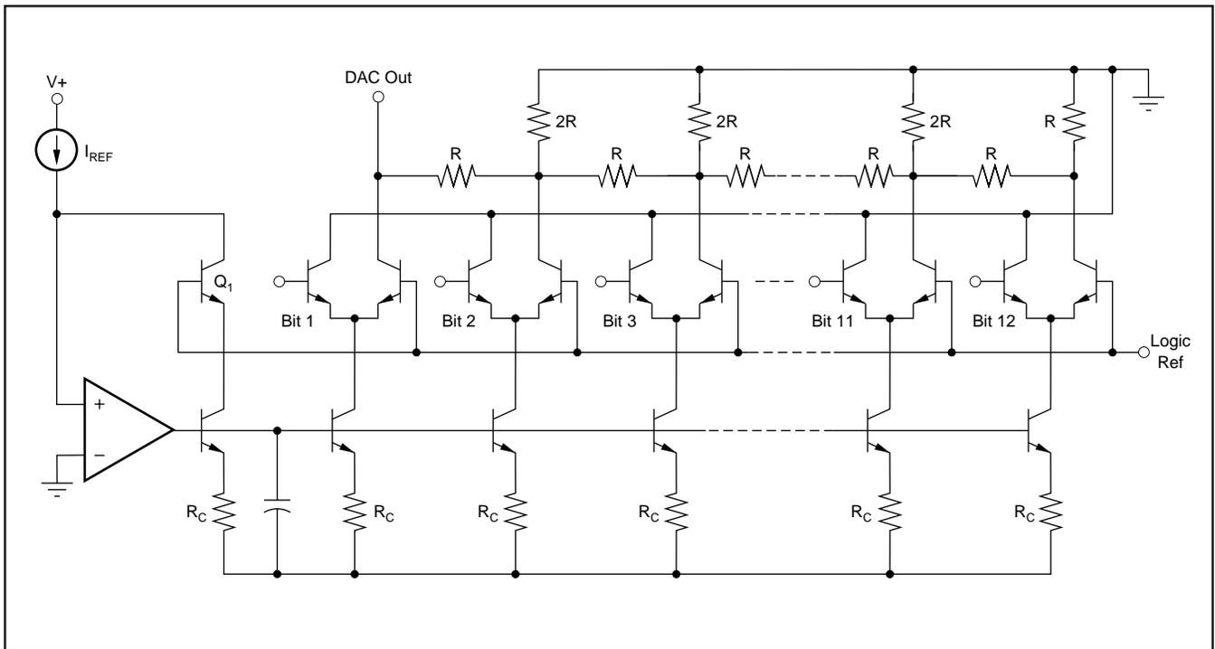
FIGURE 56. High Speed DAC with Equally Weighted Currents.
