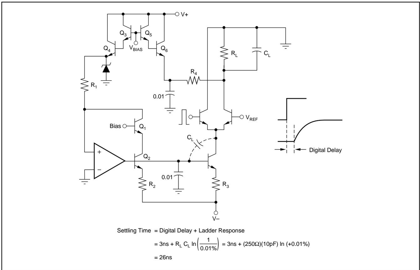
FIGURE 65. Settling Time.
