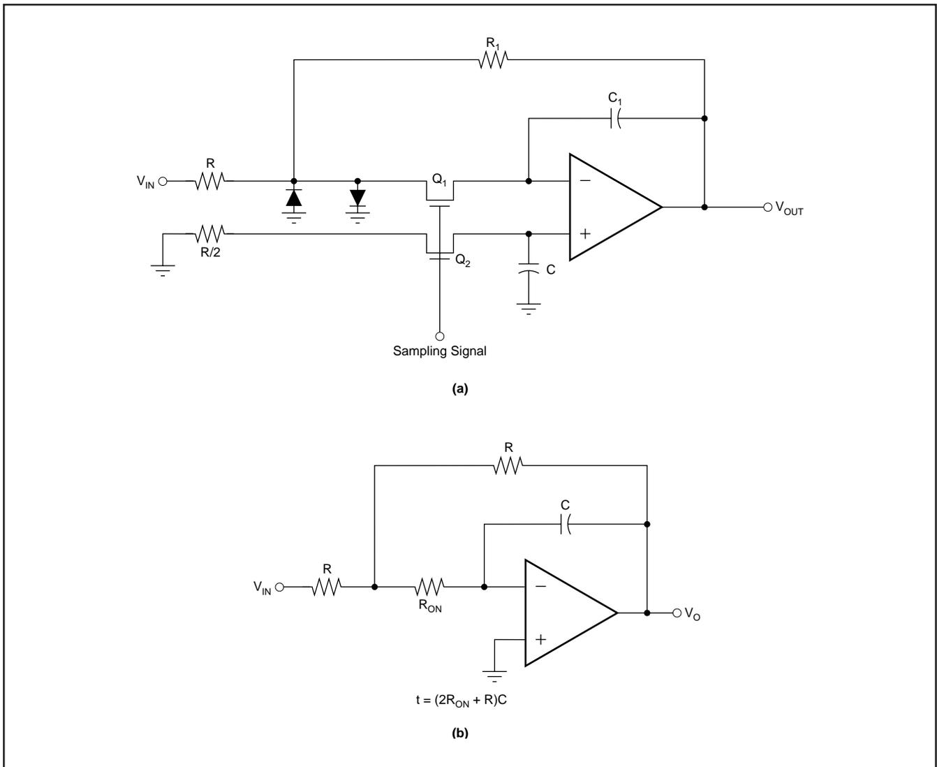
FIGURE 46. Inverting Sample/Hold.
