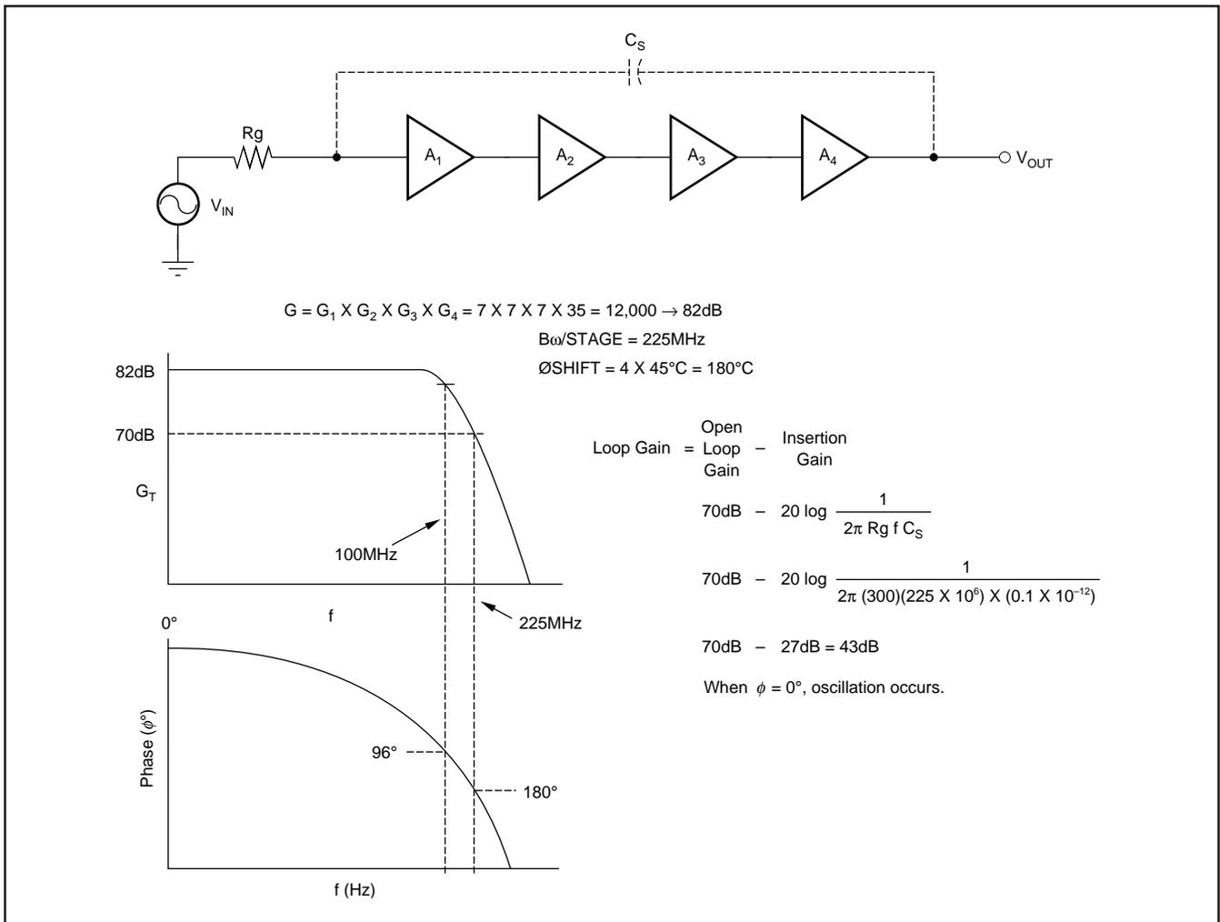
FIGURE 20. Comparator Oscillation.
