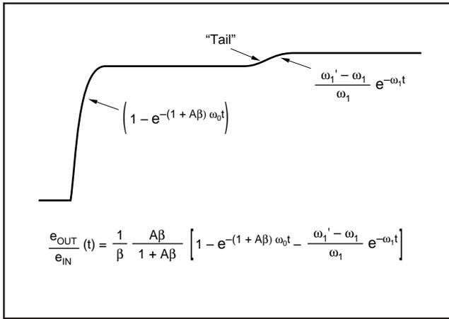
FIGURE 16. Pole-Zero Transient Response and Pole-Zero Mismatch.
