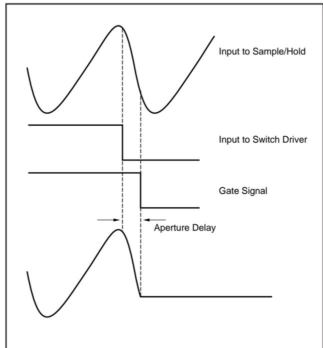
FIGURE 36. Aperture Delay.
