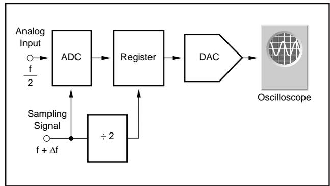
FIGURE 87. Block Diagram of Beat Frequency Tester.
