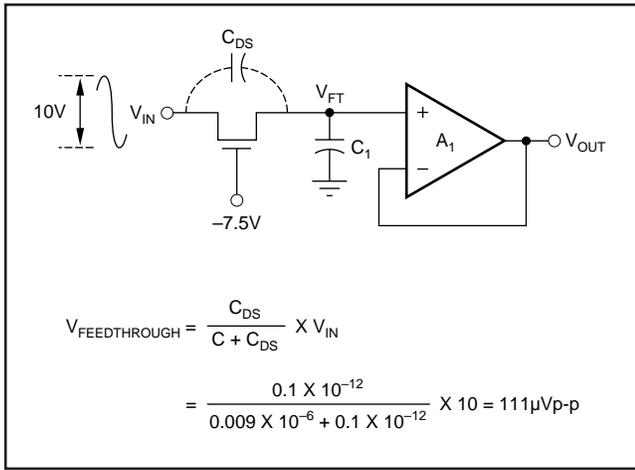
FIGURE 31. Signal Feedthrough.
