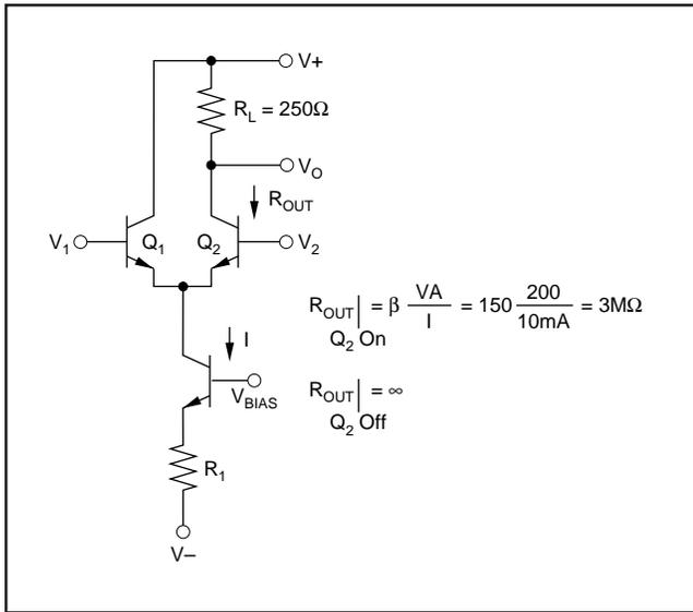
FIGURE 63. Error Due to R<sub>OUT</sub>.
