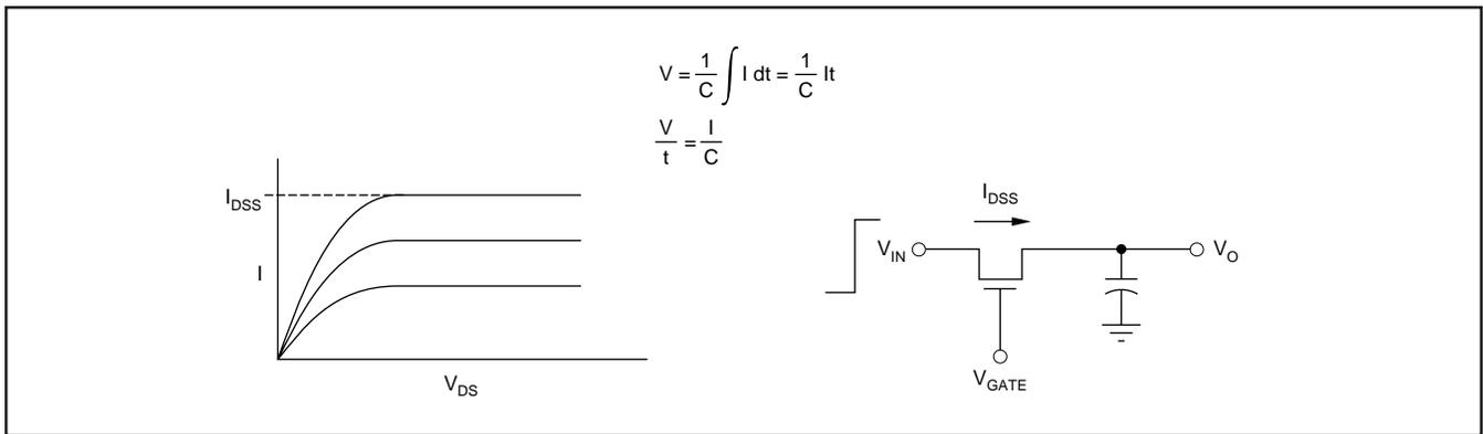
FIGURE 39. Capacitor Charged from a Constant Current.
