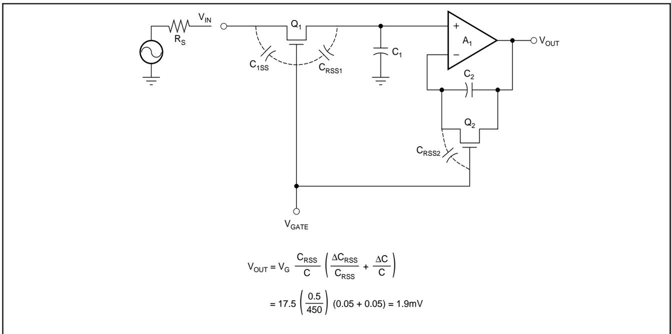
FIGURE 44. Capacitance Mismatch.
