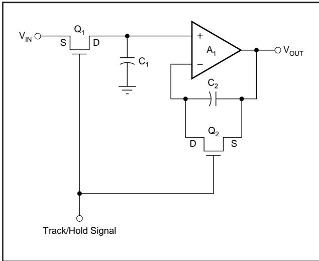
FIGURE 43. Balanced Track/Hold.
