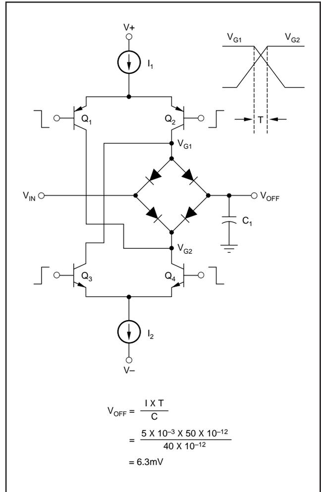
FIGURE 50. Switch Delay.
