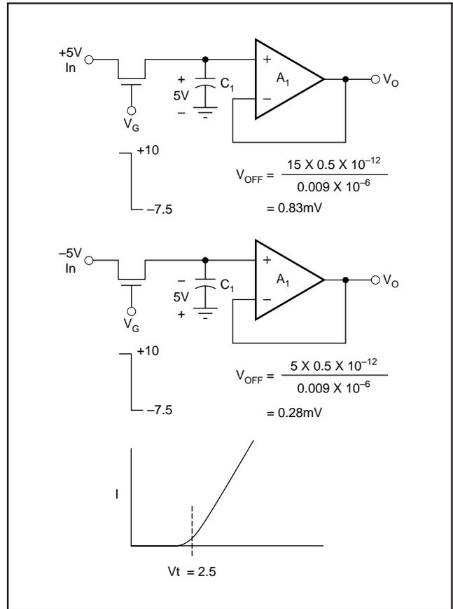
FIGURE 30. FET Threshold Characteristics and Aperture Non-linearity.
