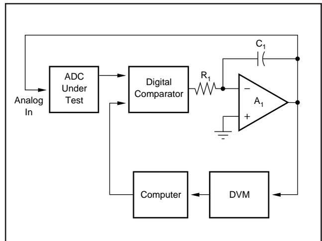
FIGURE 89. Block Diagram of Servo Loop Test.
