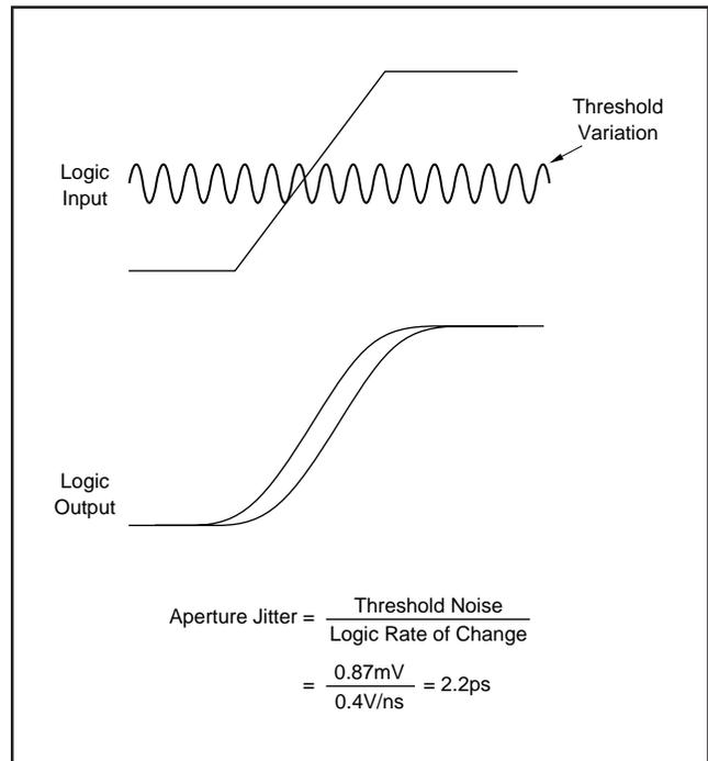
FIGURE 33. Aperture Jitter.
