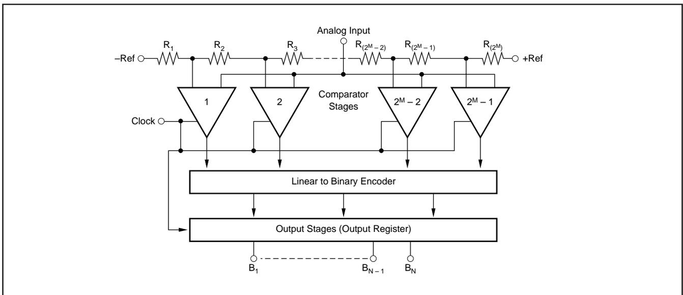
FIGURE 71. Block Diagram of a Flash Encoder.
