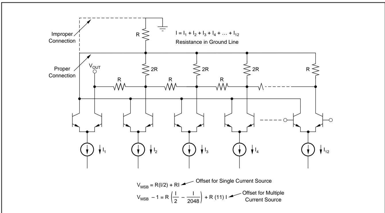
FIGURE 64. Superposition Error.
