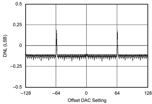
**Figure 4. DNL vs Offset DAC Setting**
