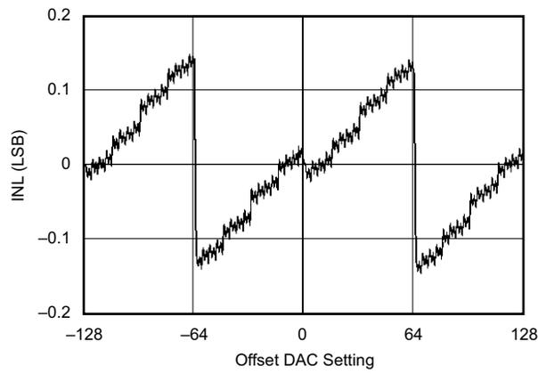
**Figure 5. INL vs Offset DAC Setting**
