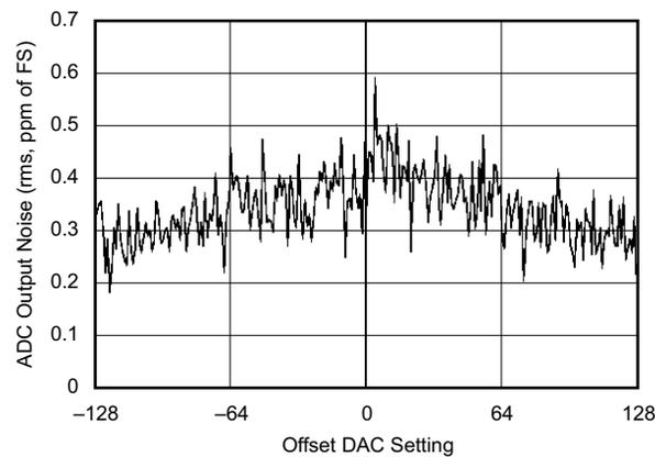
**Figure 2. ADC Output Noise vs Offset DAC Setting**
