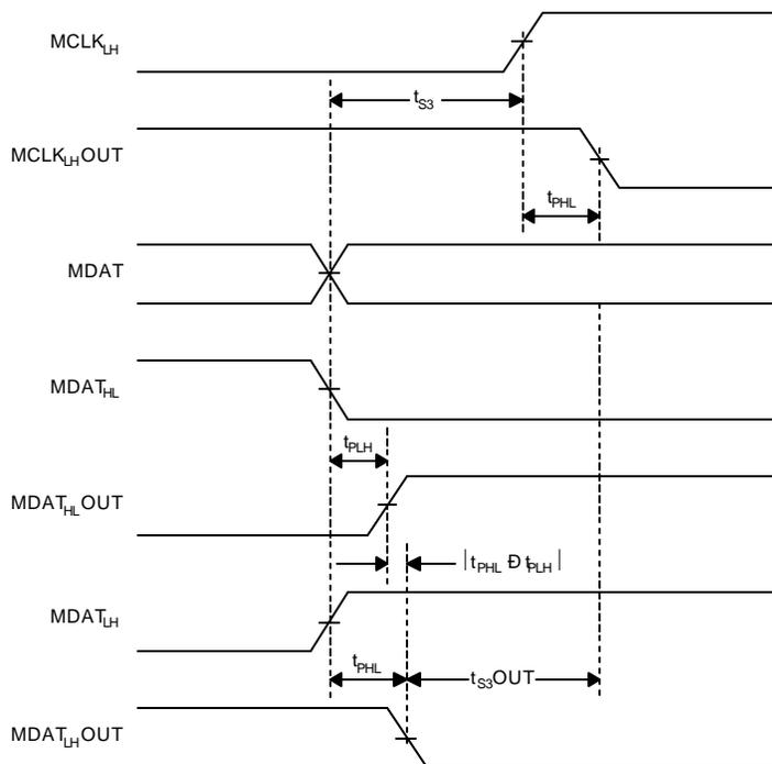
**Figure 8. Setup Time on the Rising Edge of MCLK**
