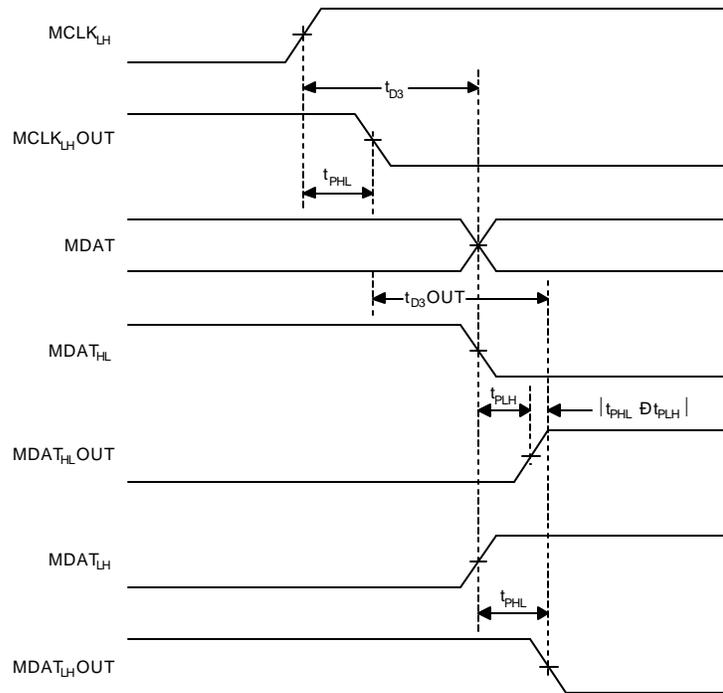
**Figure 6. Delay Time on the Rising Edge of MCLK**
