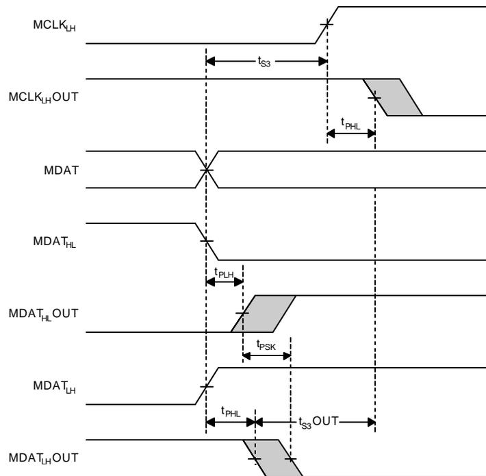
Figure 12. Setup Time on the Rising Edge of MCLK
