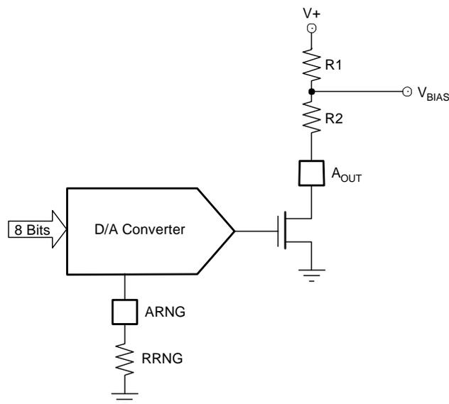
This circuit is designed for flexibility in the output voltage at the  $V_{bias}$  point shown in Figure 1 to accommodate the widely varying requirements for LCD contrast control bias.  $V_+$  can be a higher voltage than the supply voltage for the TSCs. The only restriction is that the voltage on the AOUT pin can never go above the absolute maximum rating for the device, and should stay above 1.5V for linear operation.
