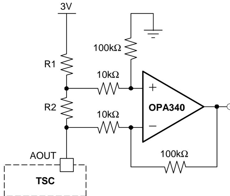
R1 and R2 must be chosen so that at the maximum DAC current, the desired output voltage, divided by the gain of the differential amplifier, is present across R2. In this example, we will assume that the maximum DAC current is 700 $\mu$ A, and that the desired output swing is 0V to 1.6V. Note that the gain in this example is 10.
