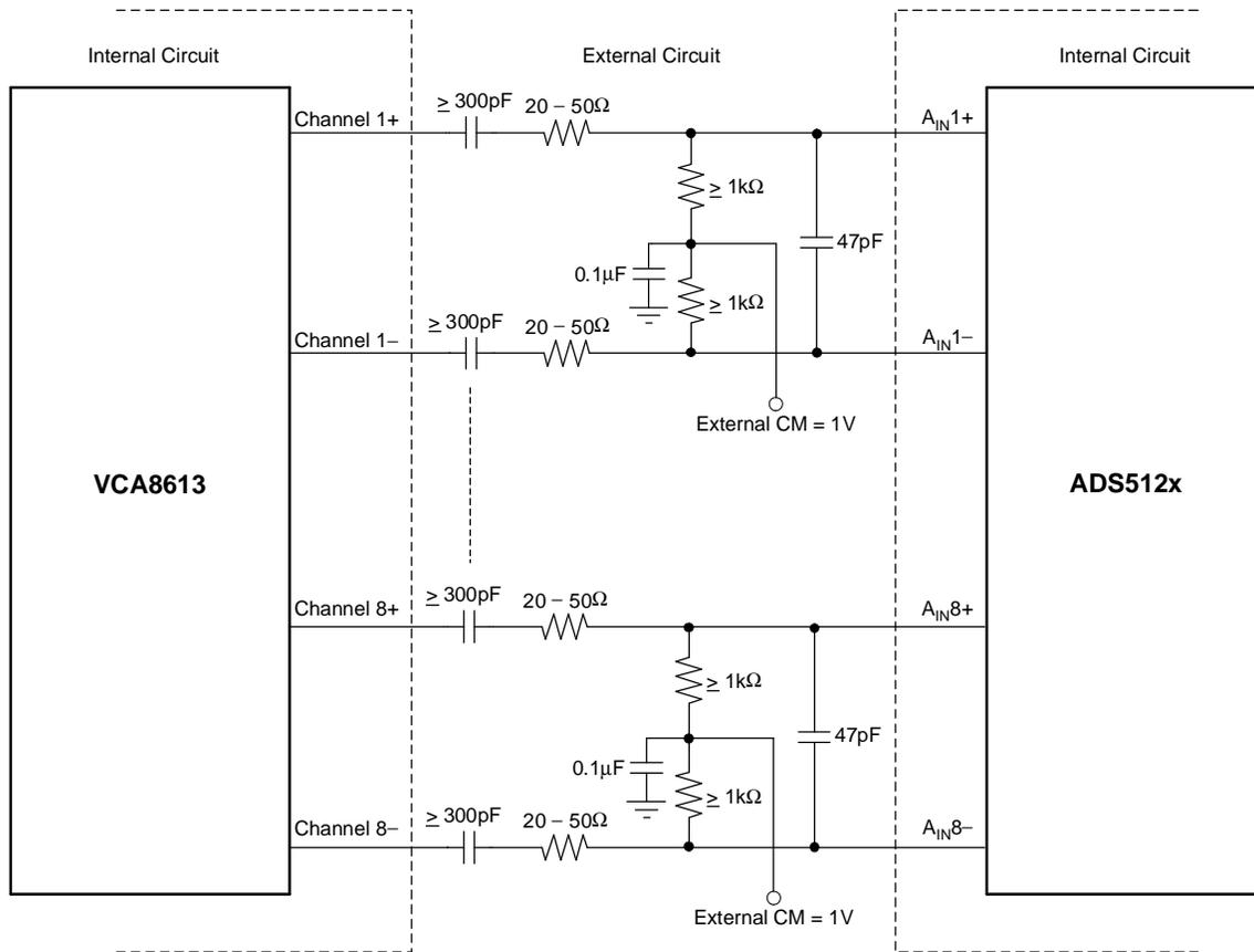
**Figure 2. AC-Coupled Interface Between VCA8613 and ADS512x**
