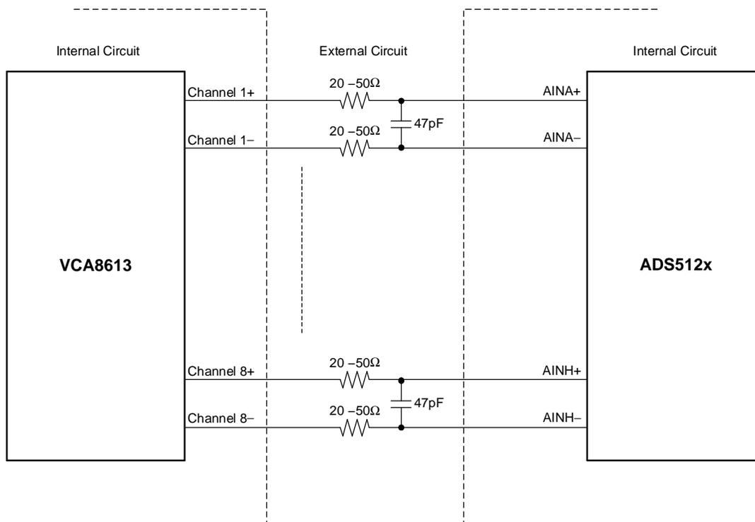
**Figure 1. DC-Coupled Interface Between VCA8613 and ADS512x**
