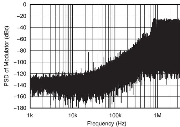
**Figure 5. Power Spectral Density of a Delta-Sigma Modulator Signal**
