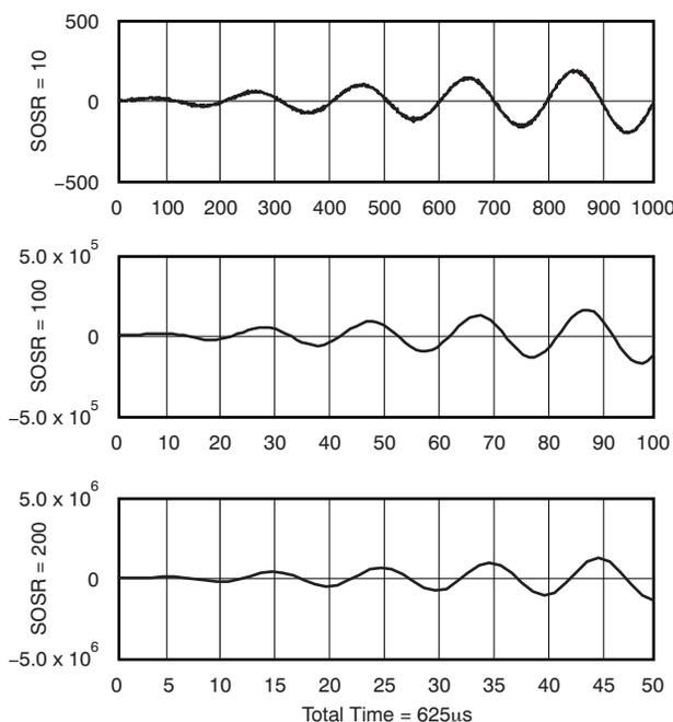
**Figure 8. Filtered Modulator Signal with Various Values of SOSR**
