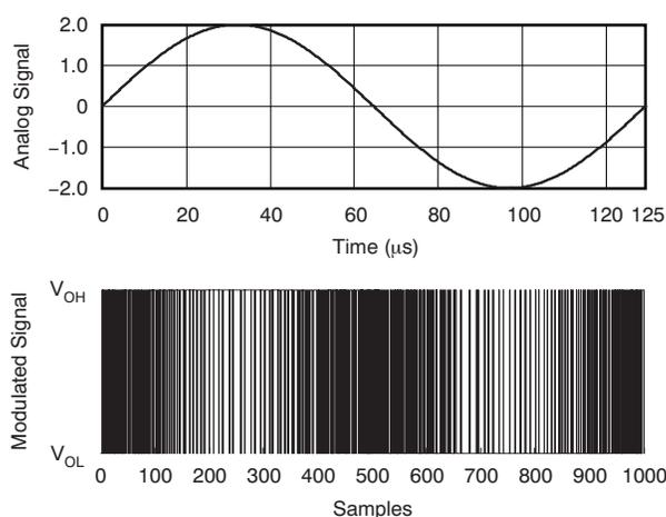
**Figure 4. Analog Input Signal and Corresponding Delta-Sigma Modulator Output**
