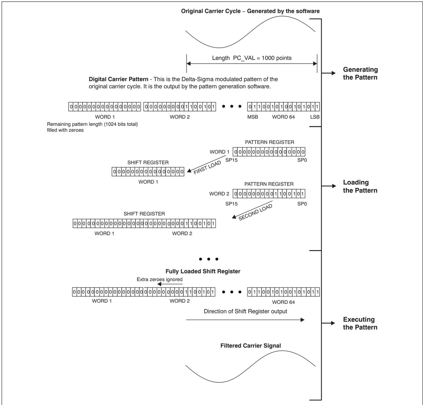
Figure 10. Loading the Pattern Register
