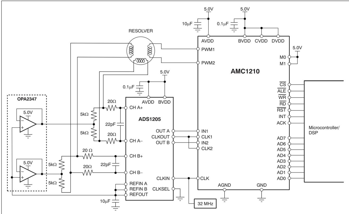
Figure 7. Typical Schematic for Resolver Application
