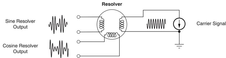
**Figure 1. Basic Resolver Diagram (with Associated Signals)**
