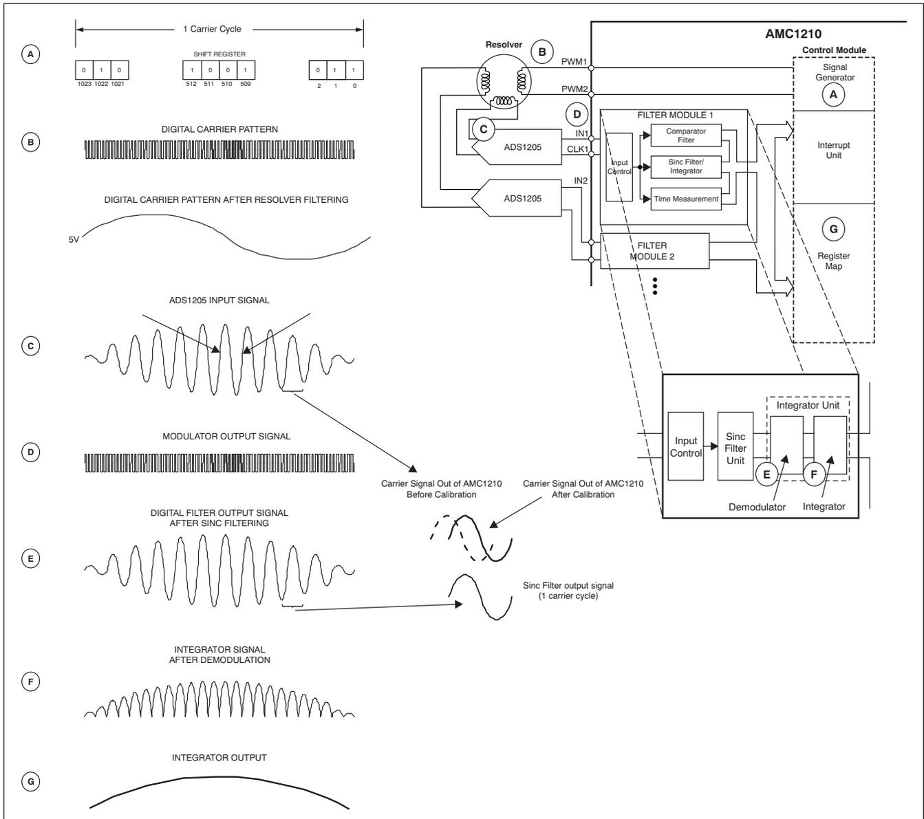
Figure 3. AMC1210 Signal Processing Sequence
