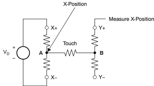
a) Add panel driving power to X+/X- pins, and read X-position from Y+ pin.
