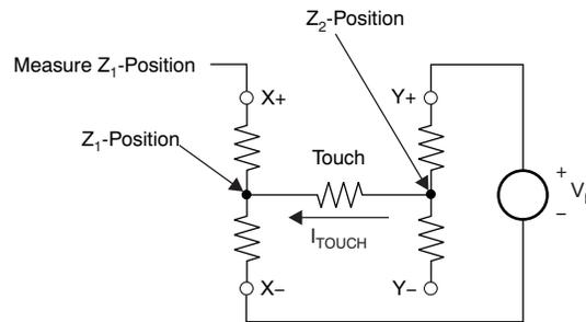
b) Add panel driving power to Y+/X- pins, and read Z<sub>1</sub>-position from X+ pin and Z<sub>2</sub>-position from Y- pin.
