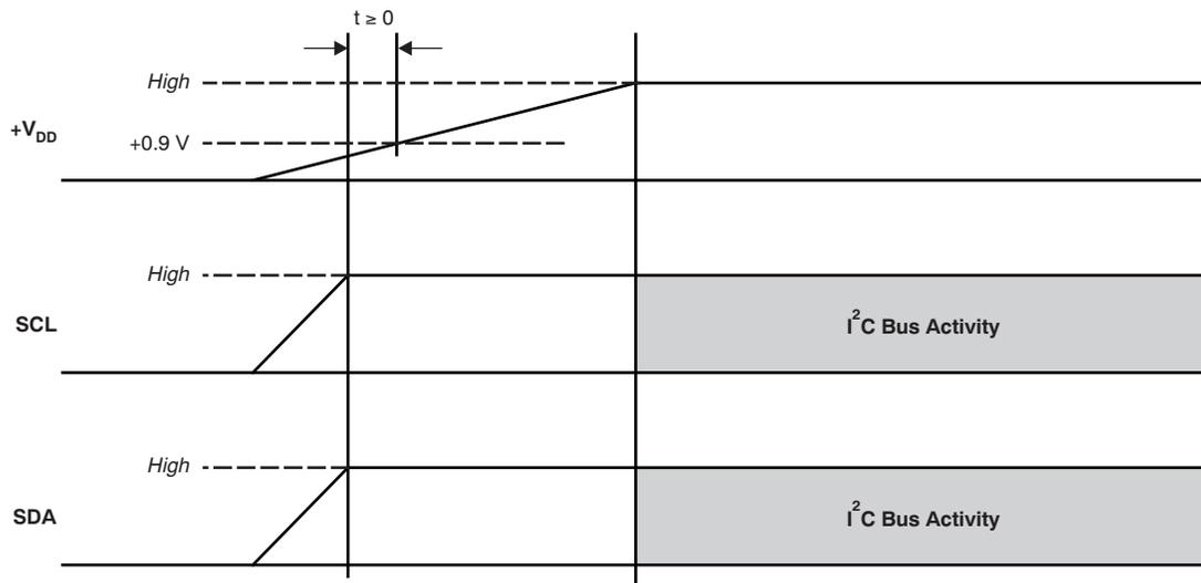
Figure 1. TSC2003 Power-Up Sequence Requirements
