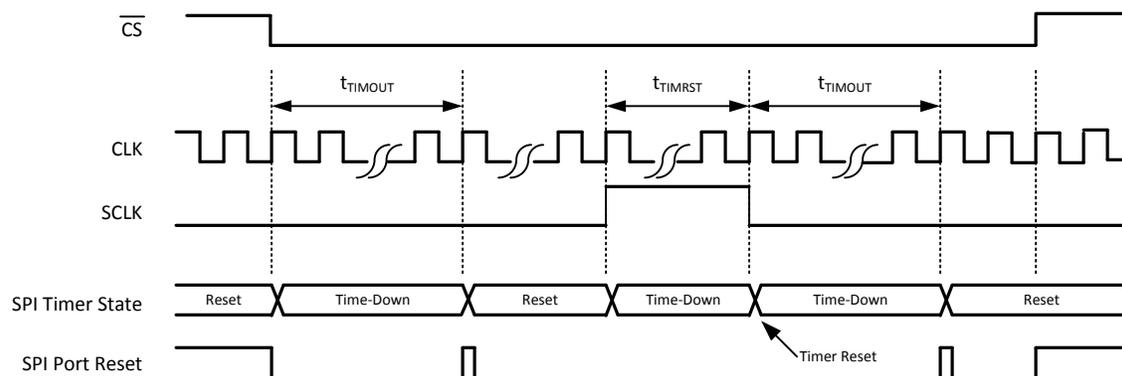
Figure 1. SPI Timeout Diagram
