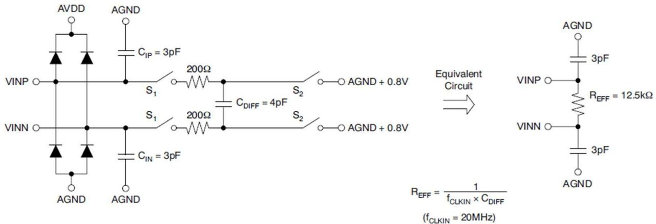
Figure 1. Equivalent Analog Input Circuit
