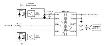
Figure 1. AMC1301 Functional Block Diagram
