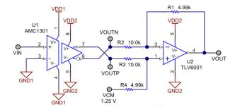
Figure 5. Scaled Differential to Single-Ended
