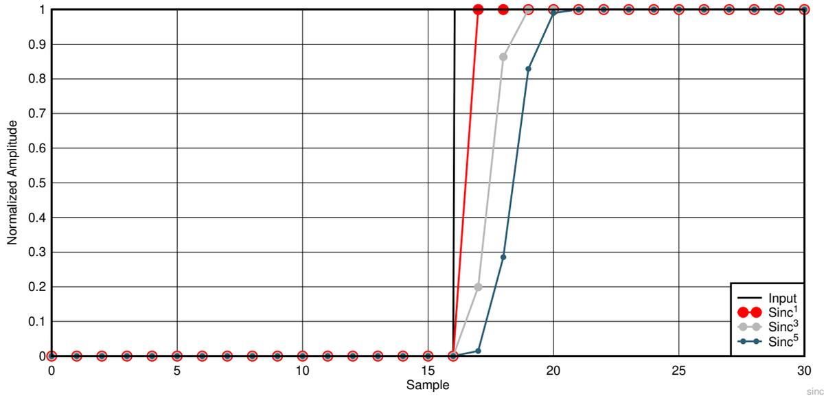
Figure 3-2. Step Response for Sinc<sup>1</sup>, Sinc<sup>3</sup>, and Sinc<sup>5</sup> Digital Filters
