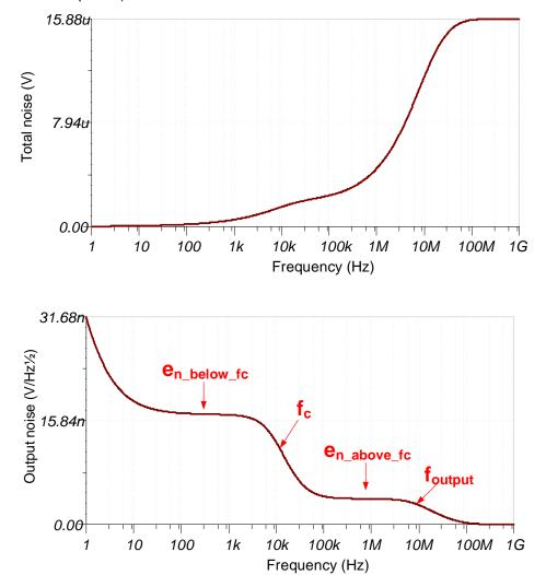
The simulated results compare well with the calculated results (that is, simulated =  $15.88\mu$ Vrms, calculated =  $14.128\mu$ Vrms).
