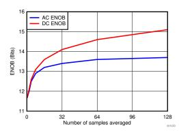
Figure 3. ENOB with ADS7x38 Programmable Averaging Filters
