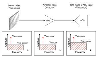
Figure 1. Noise in a Measurement System
