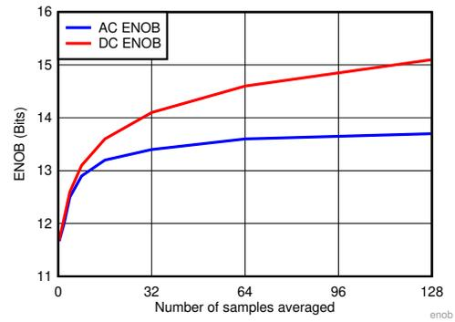
**Figure 3. ENOB with ADS7x38 Programmable Averaging Filters**
