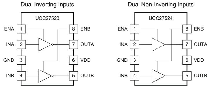
**Figure 6. UCC27523 (Inverting) and UCC27524 (Non-inverting) Block Diagrams**
