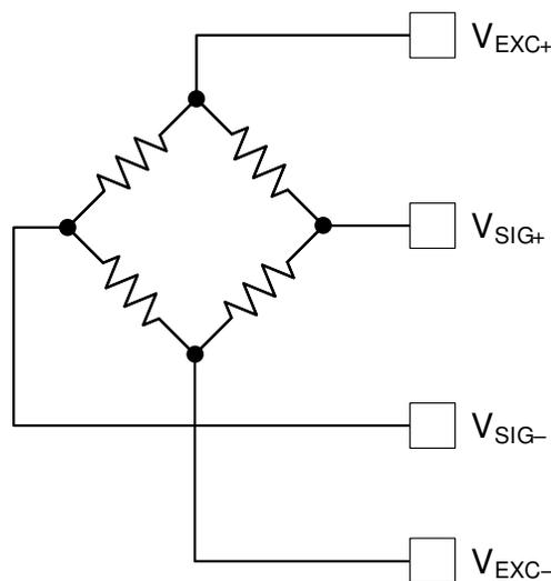
**Figure 1. Resistive Bridge in a Load Cell**
