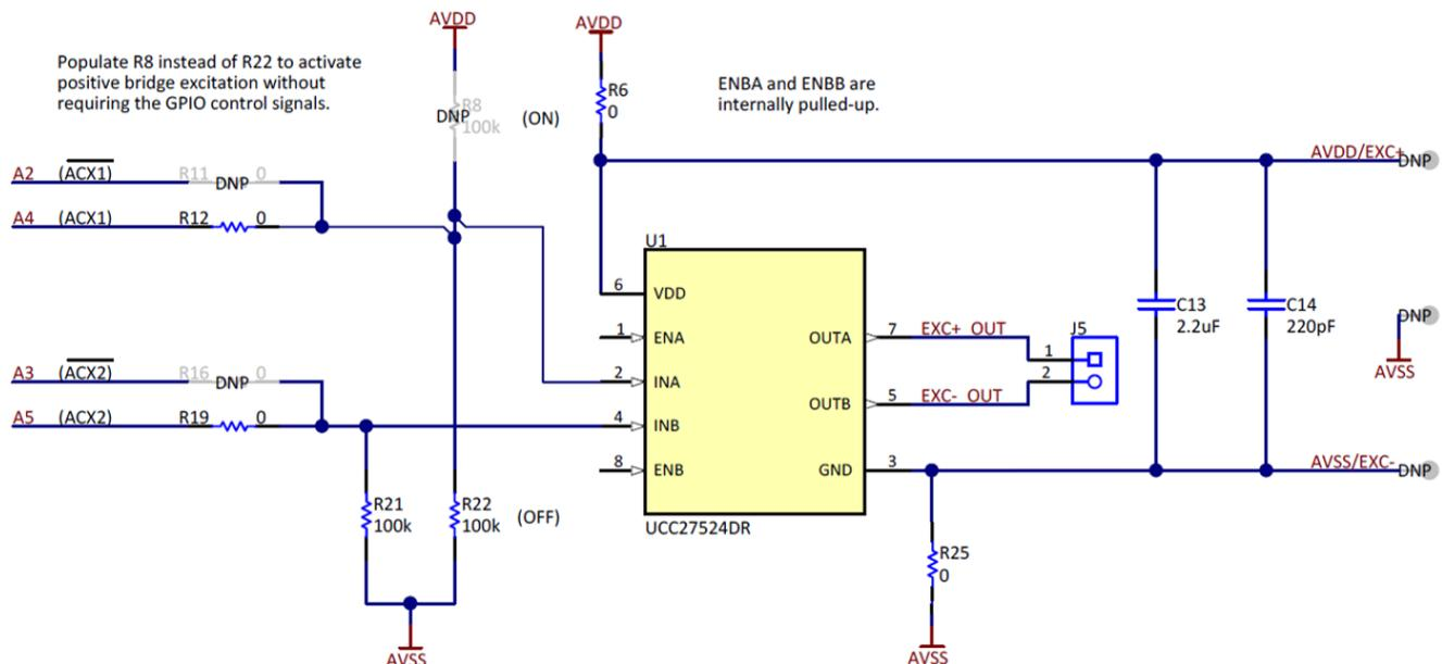
**Figure 7. AC Excitation Circuit on the ADS1235 EVM**
