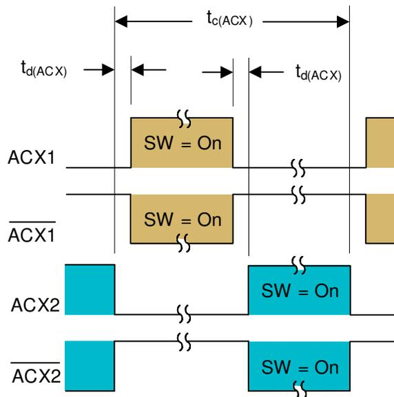
Figure 3. ADS1235 AC Excitation Signal Timing Diagram
