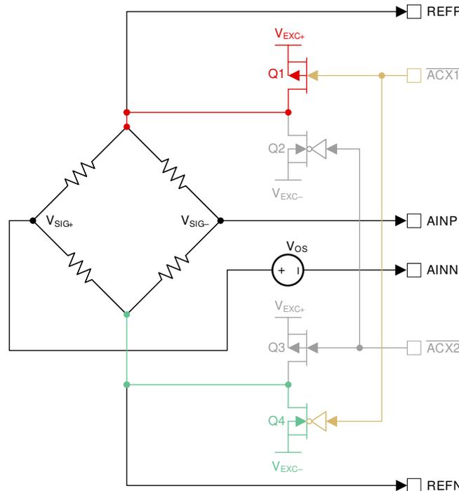
Figure 5. Phase 1 Connection Diagram for 2-Wire AC Excitation
