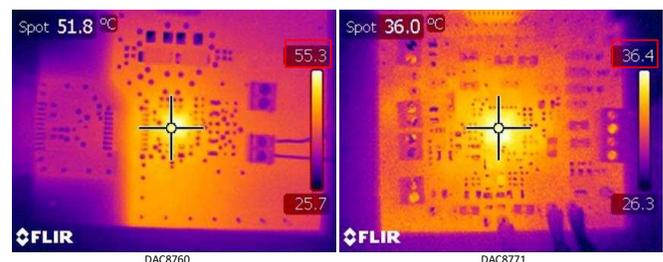
**Figure 4. Thermal Comparison of DAC8760 and DAC8771 With Adaptive Power Management**
