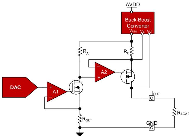
**Figure 2. 3-Wire Transmitter With Adaptive Power Management**
