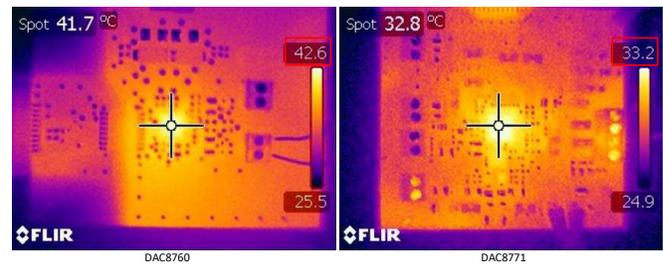
**Figure 3. Thermal Comparison of DAC8760 and DAC8771 with Adaptive Power Management**
