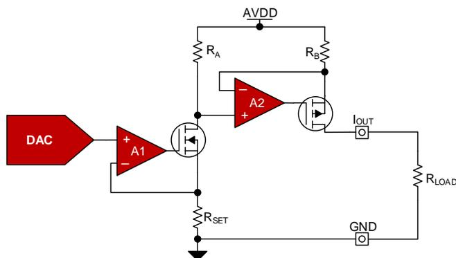
Figure 1. 3-Wire Current Transmitter Circuit
