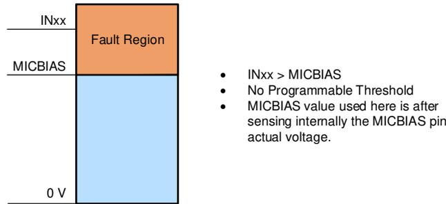
Figure 9. Input Overvoltage Conditions
