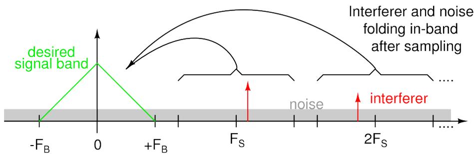
**Figure 1. Folding Back of Noise and Interferer Due to Sampling**
