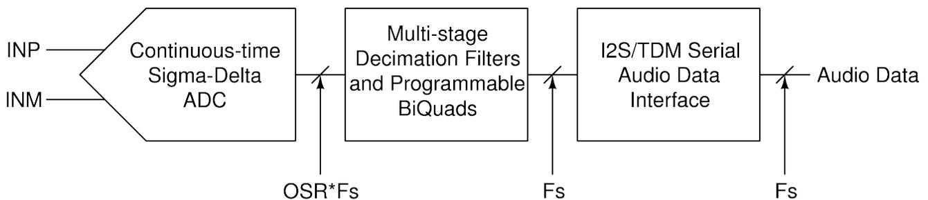
**Figure 2. Block Diagram of Audio Signal Chain**
