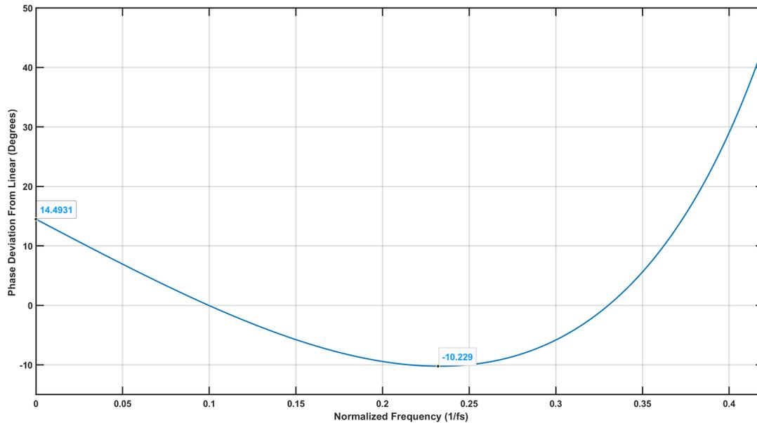
**Figure 9. Ultra-Low-Latency Decimation Filter Phase Deviation**
