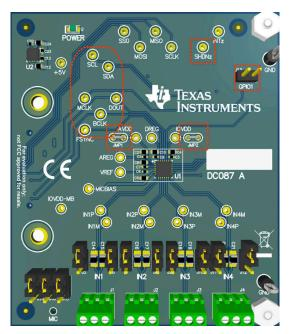
Figure 4-1. Location of TLV320ADCx140/PCMx140-Q1 EVM I<sup>2</sup>C and TDM signals
