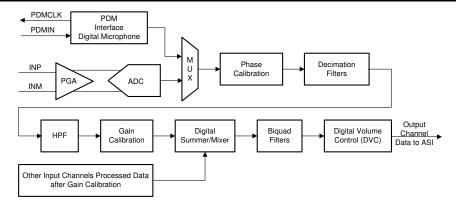
Figure 1-2. TLV320ADCx140/PCMx140-Q1 Channel Signal Chain Processing Flow Chart
