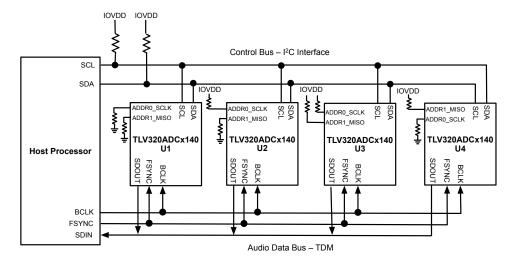
Figure 3-2. TLV320ADCx140/PCMx140-Q1 Shared TDM Connection Diagram
