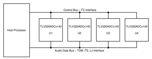
Figure 1-1. Four TLV320ADCx140/PCMx140-Q1 Devices With Shared Control and Audio Data Buses
