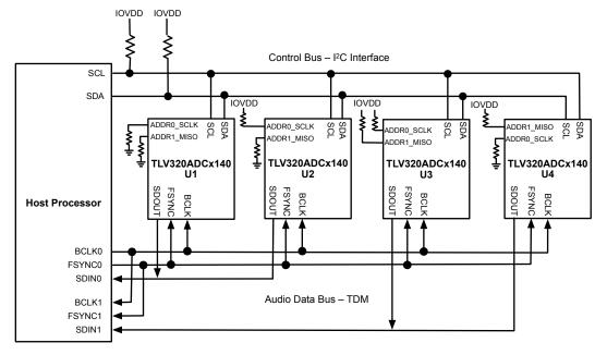
Figure 3-10. TLV320ADCx140/PCMx140-Q1 Shared Split TDM Connection Diagram
