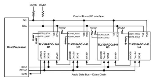
Figure 3-12. TLV320ADCx140/PCMx140-Q1 Daisy Chain TDM Connection Diagram
