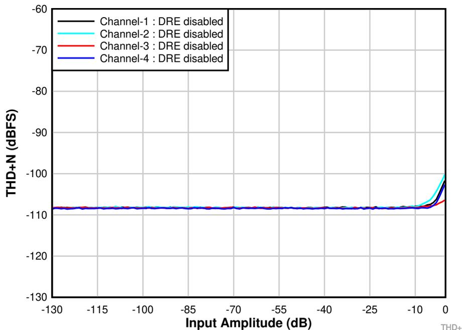
Figure 5-3. THD+N Performance Measurement with DRE Disabled
