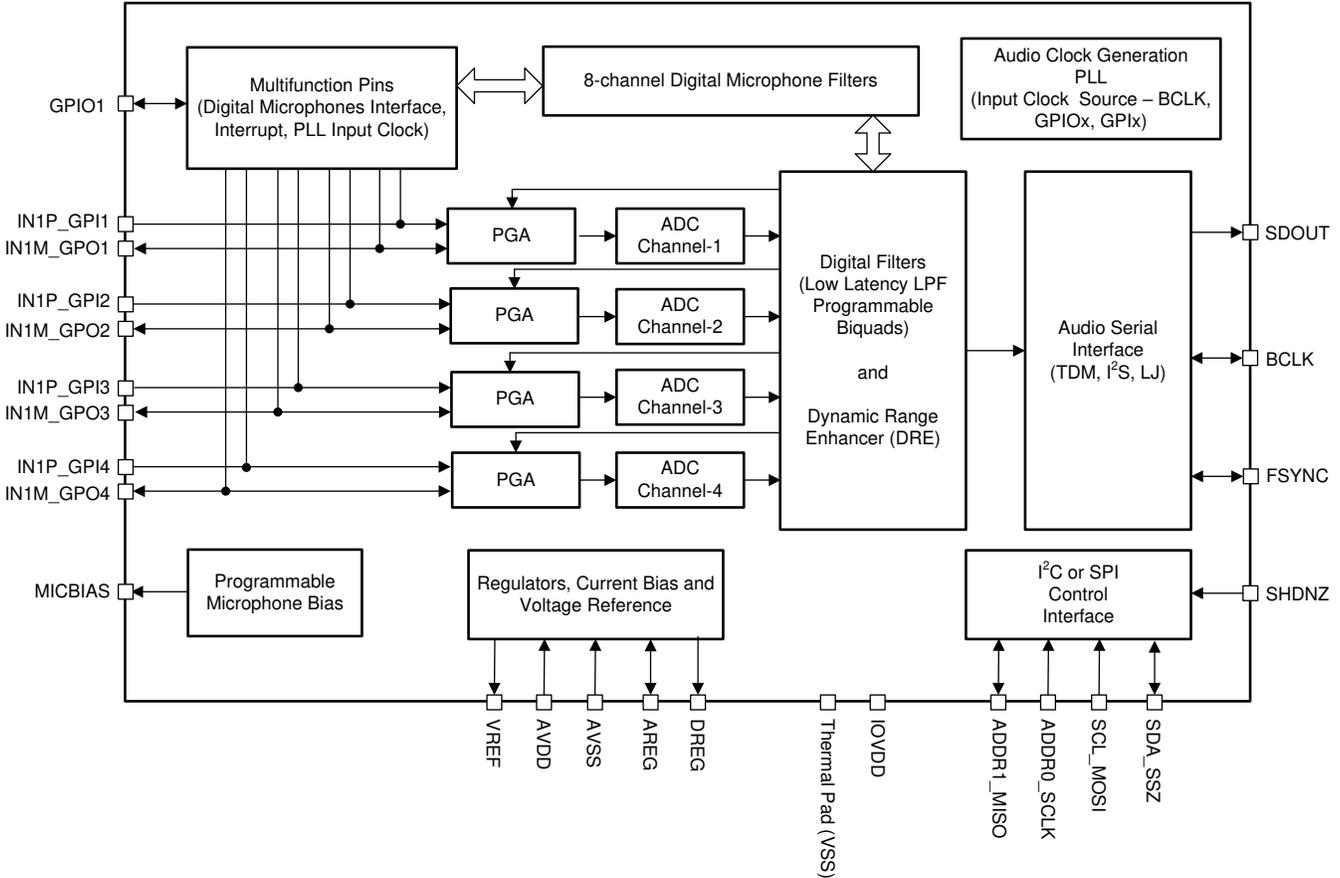
**Figure 6-1. Internal Block Diagram of the TLV320ADC5140**
