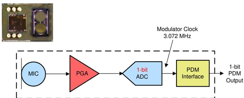
Figure 3-1. Digital PDM Microphone for 1-bit Output
