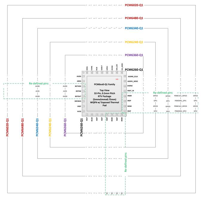
Figure 2-1. PCM6xx0-Q1 Pin-Compatibility Diagram
