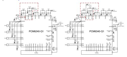
Figure 2-2. Schematic Differences Between PCM6240-Q1 and PCM6340-Q1
