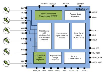
Figure 1-1. PCM6260-Q1 Functional Block Diagram
