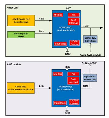
Figure 4-5. ANC in Standalone Module, Hands-free Beamforming and AUXIN or Voice input in Head-unit
