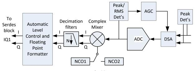
Dual NCOs Figure 3. AFE7920 Receiver Single DDC Block Diagram
