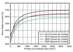
Figure 1. Shunt Rated Current vs PCB Size
