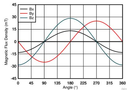
Figure 2. Magnetic Flux Density vs Magnet Angle
