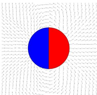
Figure 1. Diametric Magnet
