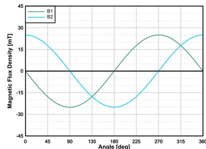
Figure 3. Field Components With  $90^\circ$  Phase Shift
