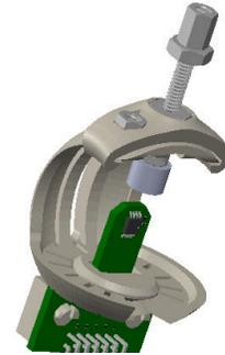
**Figure 4. TMAG5170 Orbital Attachment**
