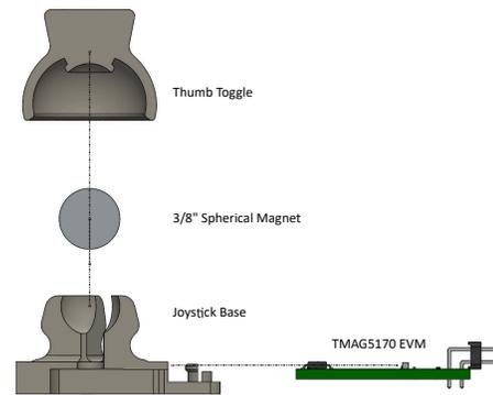
**Figure 7. Thumb Toggle Joystick Exploded View**
