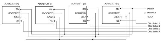
Figure 6. Conventional SPI Cascade Connection
