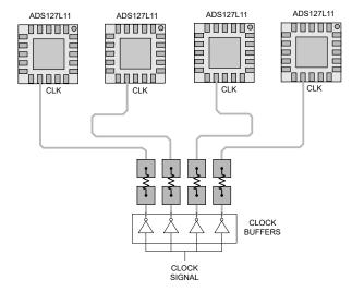
Figure 2. Multiple Clock Buffers
