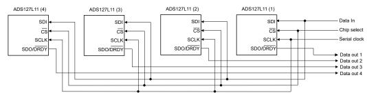
Figure 10. Parallel SDO/DRDY Connection
