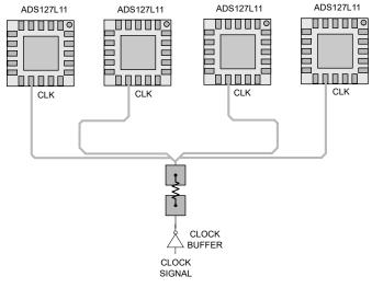
Figure 1. Single Clock Buffer
