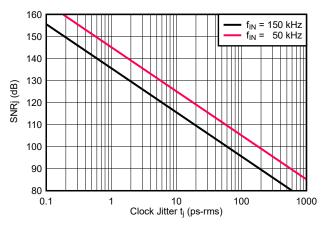
Figure 3. SNR<sub>i</sub> vs. Clock Jitter
