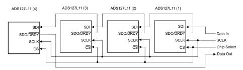
Figure 7. Daisy-Chain SPI Connection
