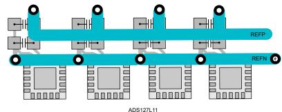
Figure 11. Reference Voltage Routing
