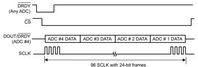
Figure 9. Daisy-Chain Data Output Sequence
