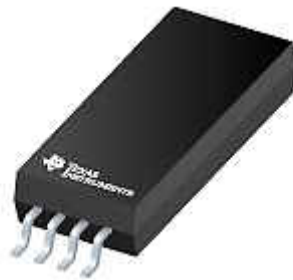
Figure 3. DWL Package, 8-Pin SOIC
