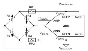
Figure 3-3. Four-Wire Bridge With Parasitic Resistance in V<sub>EXCITATION±</sub> Leads
