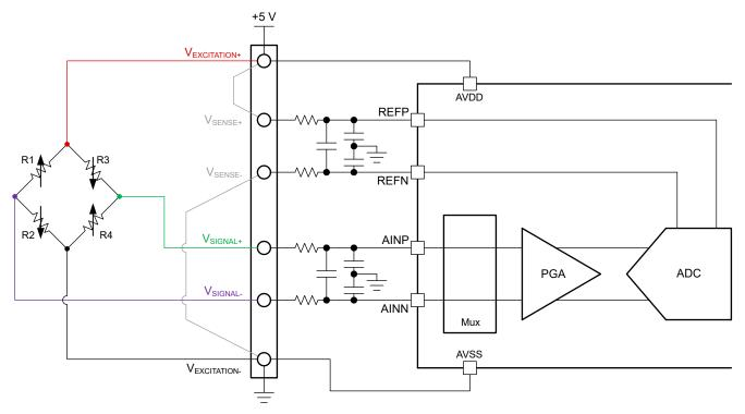
Figure 6-1. Four-Wire Resistive Bridge Measurement with a Ratiometric Reference and a Unipolar, Low-Voltage (≤ 5 V) Excitation Source
