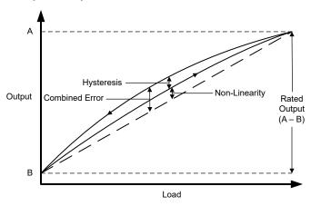
Figure 4-2. Hysteresis, Non-Linearity, and Combined Error
