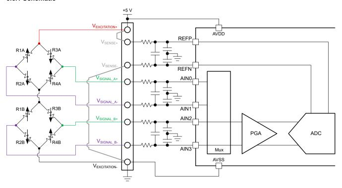
Figure 6-11. Measuring Multiple Four-Wire Resistive Bridges in Series With a Pseudo-Ratiometric Reference and a Unipolar, Low-Voltage (≤ 5 V) Excitation Source
