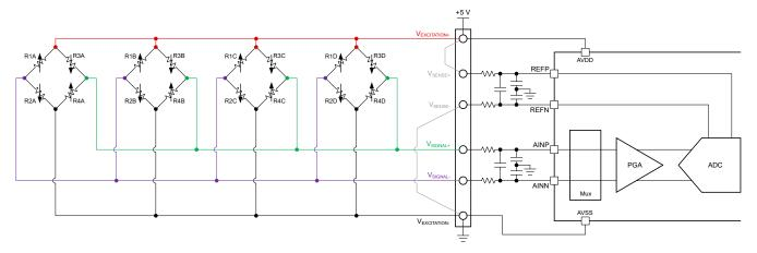
Figure 6-14. Measuring Multiple Four-Wire Resistive Bridges in Parallel Using a Single-Channel ADC With a Ratiometric Reference and a Unipolar, Low-Voltage (≤ 5 V) Excitation Source
