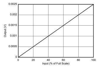
Figure 2-2. Quarter Bridge Differential Output (R = 1 k $\Omega$ , V<sub>EXCITATION</sub> = 10 V,  $\Delta$ R<sub>FS</sub> = 1  $\Omega$ )
