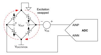
Figure 5-10. Bridge Measurement During AC Excitation (Phase 2)
