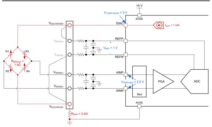
Figure 6-10. Current-Excited Bridge Measurement Using  $R_{BRIDGE}$  = 1 k $\Omega$ ,  $R_{BIAS}$  = 2 k $\Omega$ , and  $I_{IDAC}$  = 1 mA
