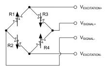
Figure 3-2. Connections for a Four-Wire Bridge
