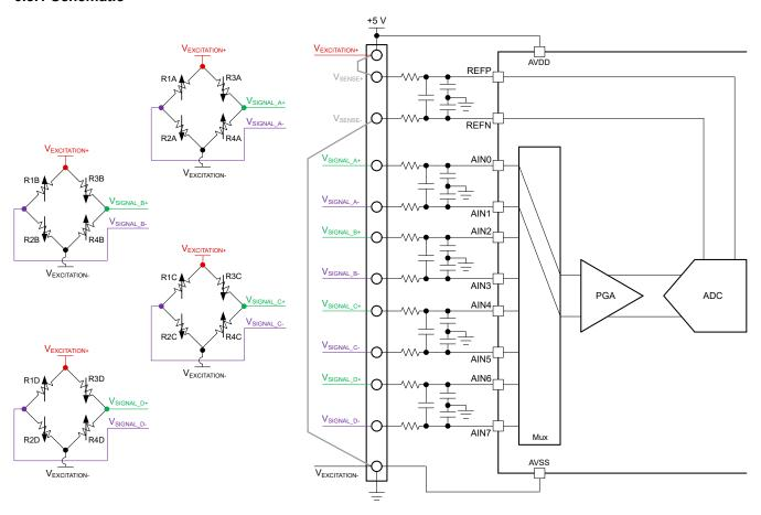
Figure 6-19. Measuring Multiple Four-Wire Resistive Bridges in Parallel Using a Multichannel ADC With a Ratiometric Reference and a Unipolar, Low-Voltage (≤ 5 V) Excitation Source
