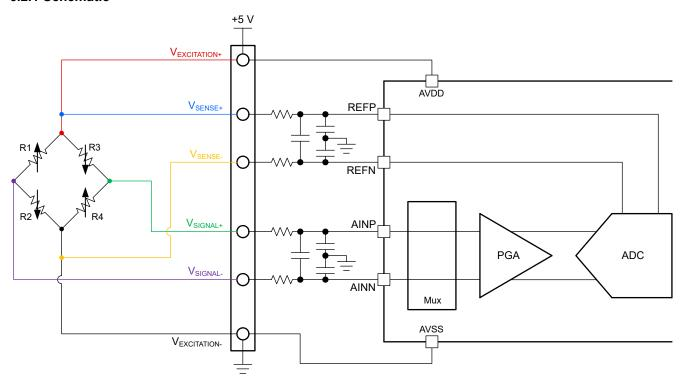
Figure 6-2. Six-Wire Resistive Bridge Measurement With a Ratiometric Reference and a Unipolar, Low-Voltage (≤ 5 V) Excitation Source
