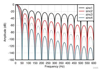
Figure 5-6. ADS1235 Sinc Filter Frequency Responses at ODR = 50 SPS
