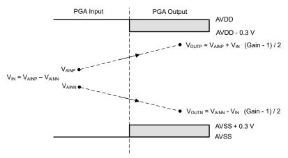
Figure 5-4. Graphical Representation of the ADS1235 PGA Input and Output Range
