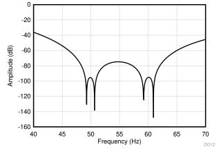
Figure 5-8. ADS1235 FIR Frequency Response
