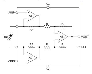
Figure 5-1. Topology of a Basic INA
