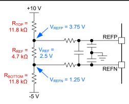
Figure 6-6. Example Resistor and Voltage Values
