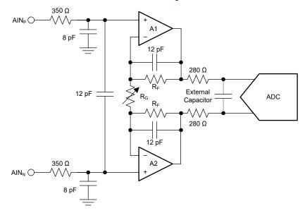
Figure 5-3. Simplified ADS1235 PGA Diagram
