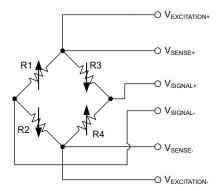
Figure 3-4. Connections for a Six-Wire Bridge
