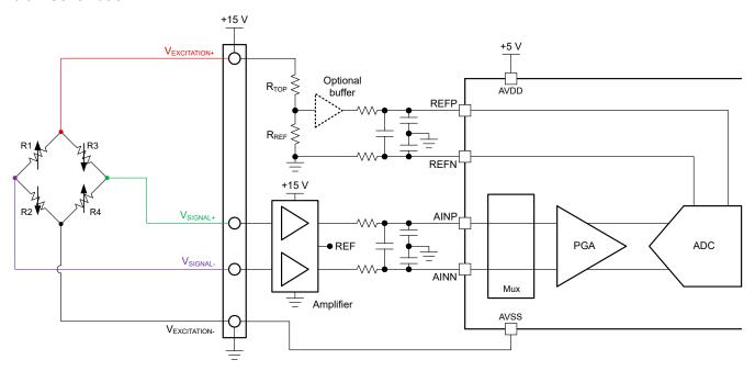
Figure 6-3. Four-Wire Resistive Bridge Measurement With a Pseudo-Ratiometric Reference and a Unipolar, High-Voltage (> 5 V) Excitation Source
