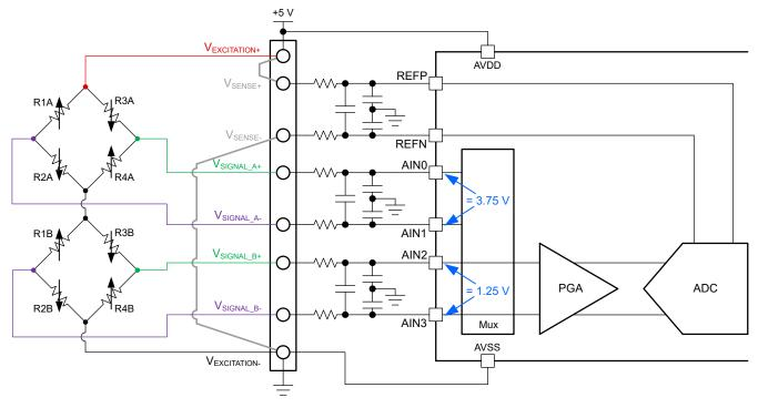
Figure 6-12. Common-Mode Voltage for Two Bridges in a Series Configuration
