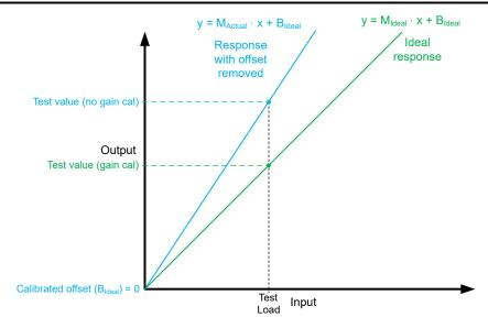
Figure 5-14. Gain Calibration Calculates the Scaling Factor (MACTUAL) from the Test Load
