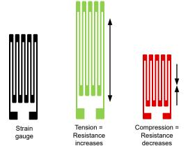
Figure 2-9. Strain Gauge Resistance vs Length: Resting (left), Tension (middle), and Compression (right)
