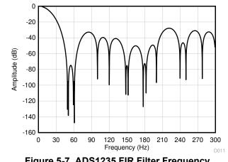
Figure 5-7. ADS1235 FIR Filter Frequency Response at ODR = 20 SPS
