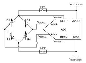
Figure 3-5. Six-Wire Bridge With Parasitic Resistance in V<sub>EXCITATION±</sub> Leads
