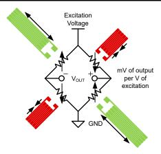
Figure 2-12. Equivalent Bridge Measurement of the Load Cell
