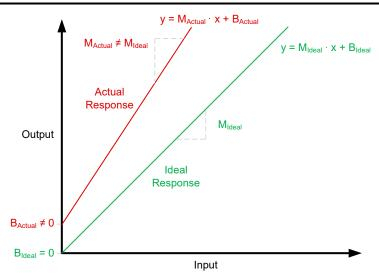
Figure 5-11. Bridge Measurement Response: Ideal vs Actual
