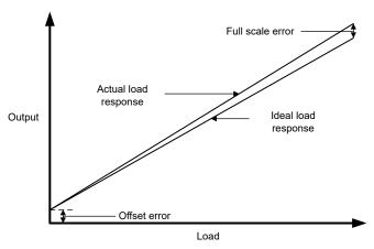
Figure 4-1. Actual vs Ideal Response of a Load on a Bridge
