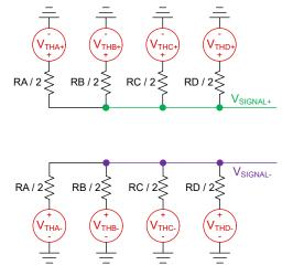
Figure 6-16. Thevenin Equivalent of Four Bridge Circuits in Parallel
