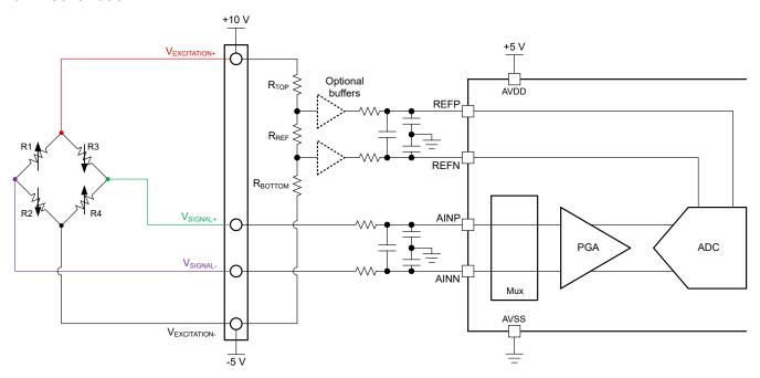
Figure 6-5. Four-Wire Resistive Bridge Measurement With a Pseudo-Ratiometric Reference and Asymmetric, High-Voltage (> 5 V) Excitation Source
