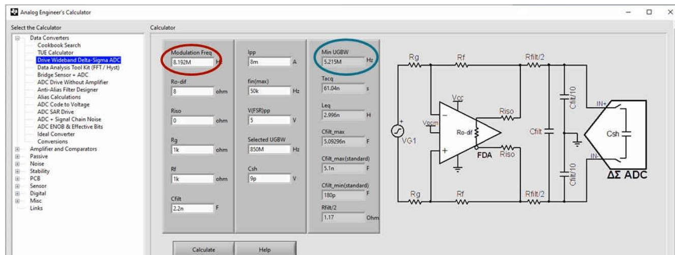
The calculator interface shows the **Modulation Freq** set to **8.192M** Hz. The **Min UGBW** is calculated as **5.215M** Hz. The right side shows the **Reference Schematic** for the **ΔΣ ADC** circuit.
