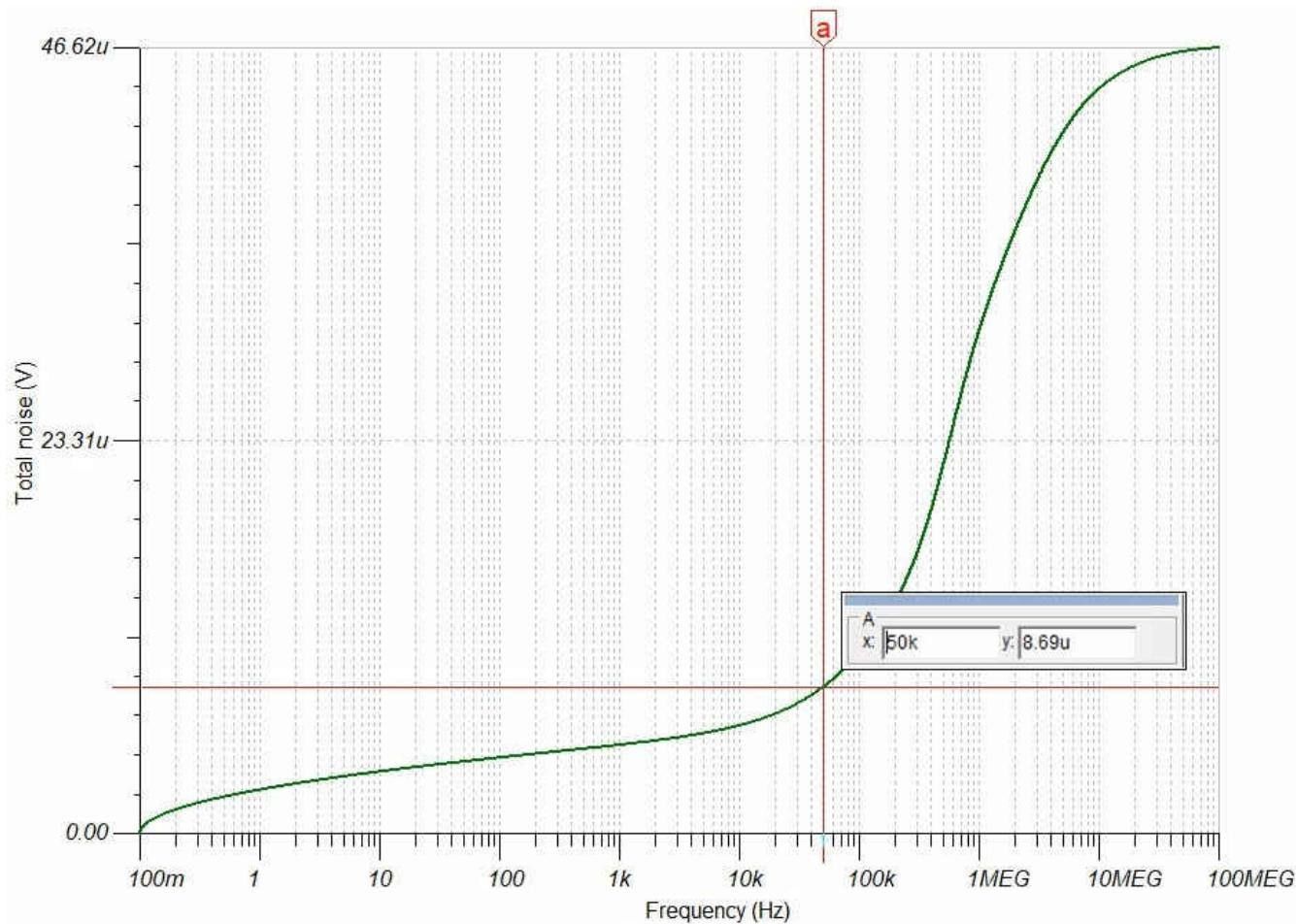
**Figure 2-6. Total Noise Result of the Analog Input Circuit to the ADC**
