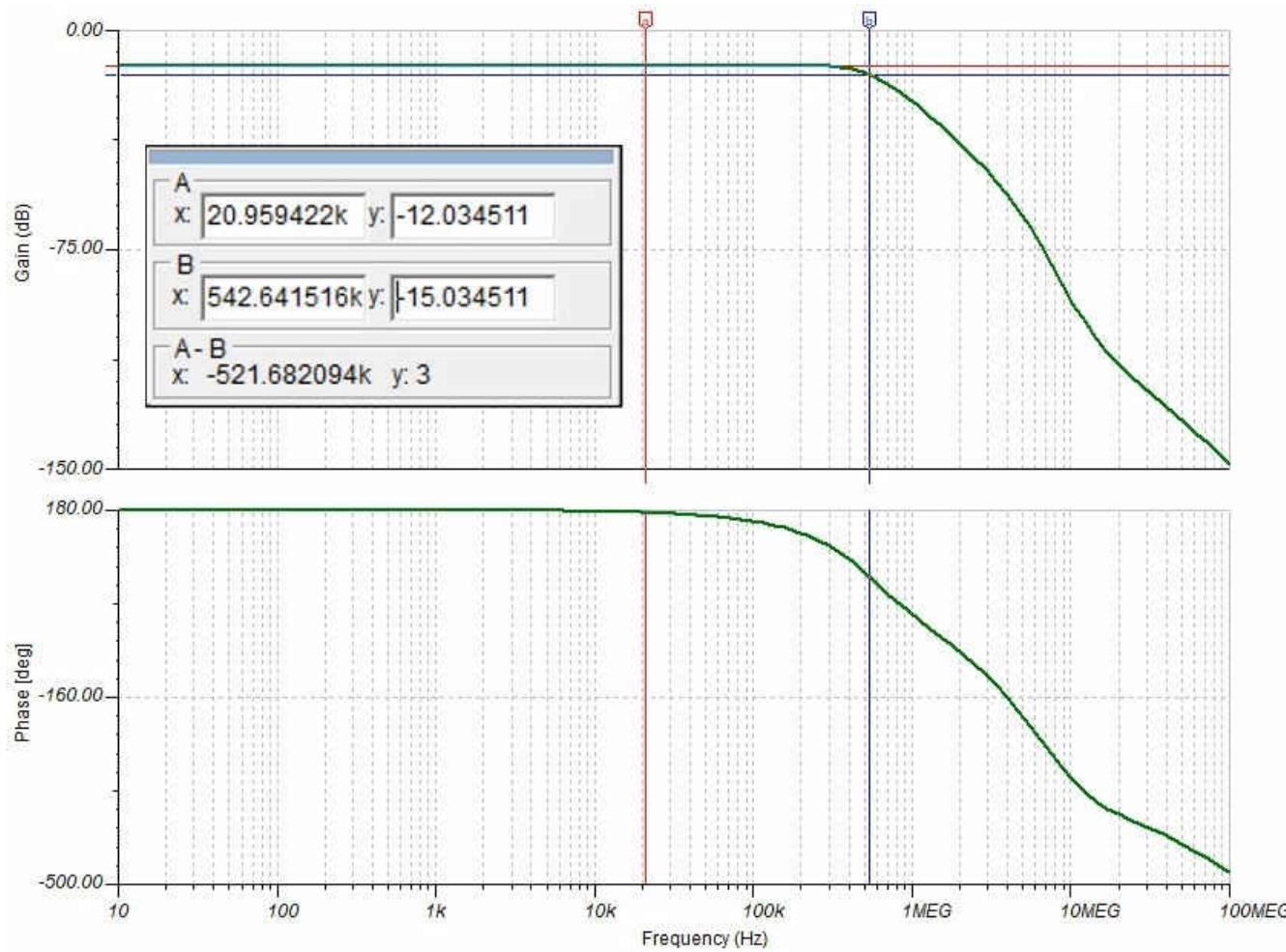
**Figure 2-9. AC Transfer Characteristic of Analog Front End – 3 dB Bandwidth of VOUTdiff is 542.96 kHz**
