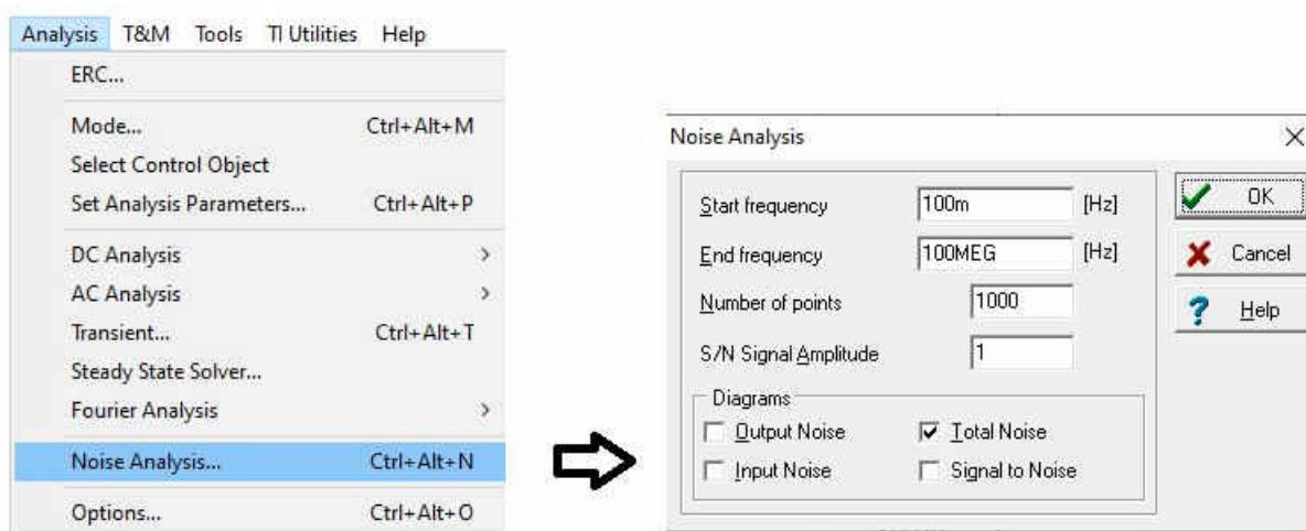
**Figure 2-5. Select ‘Noise Analysis’ and Check ‘Total Noise’ in Tina-TI Simulator**
