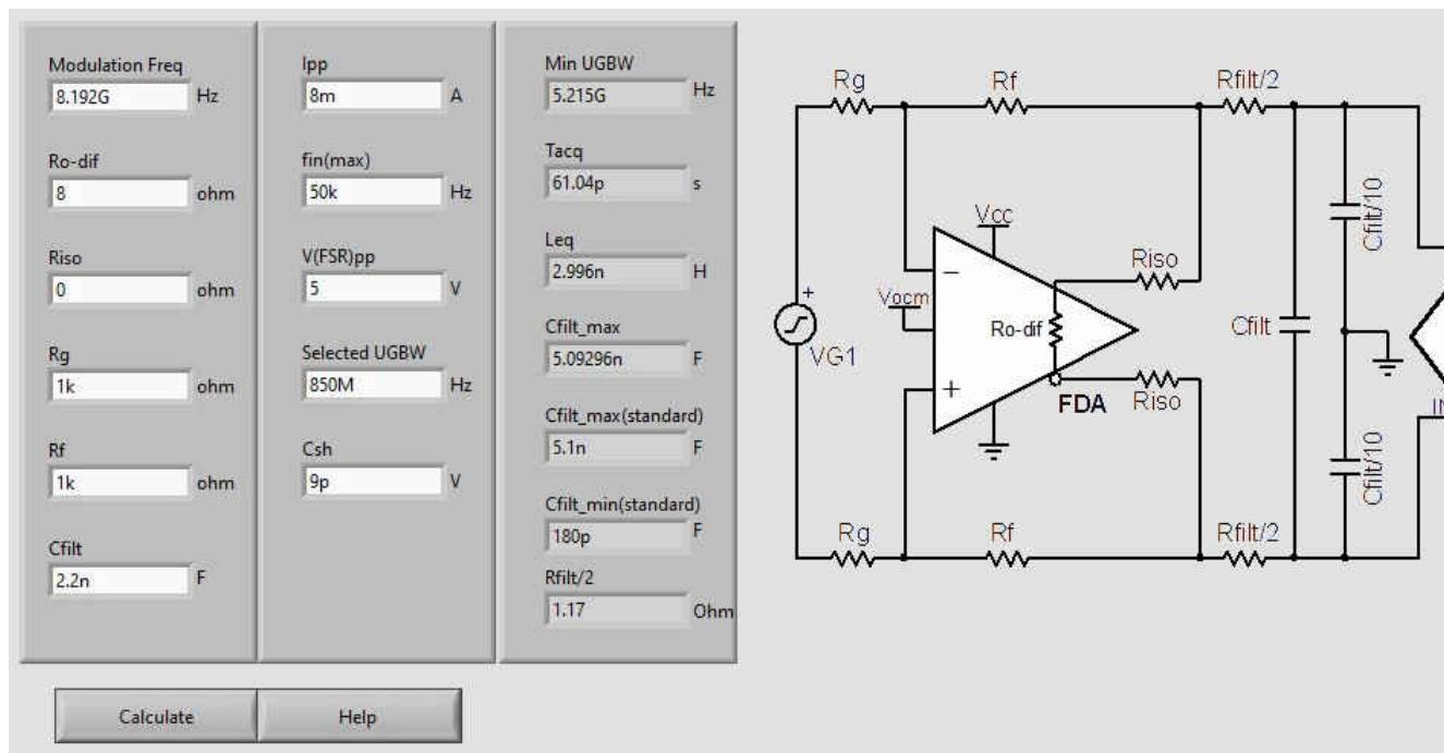
**Figure 1-6. User Defined And Calculated Values For The Reference Schematic With LMH5485-SP and ADS1278-SP to Meet the Example Design Targets**
