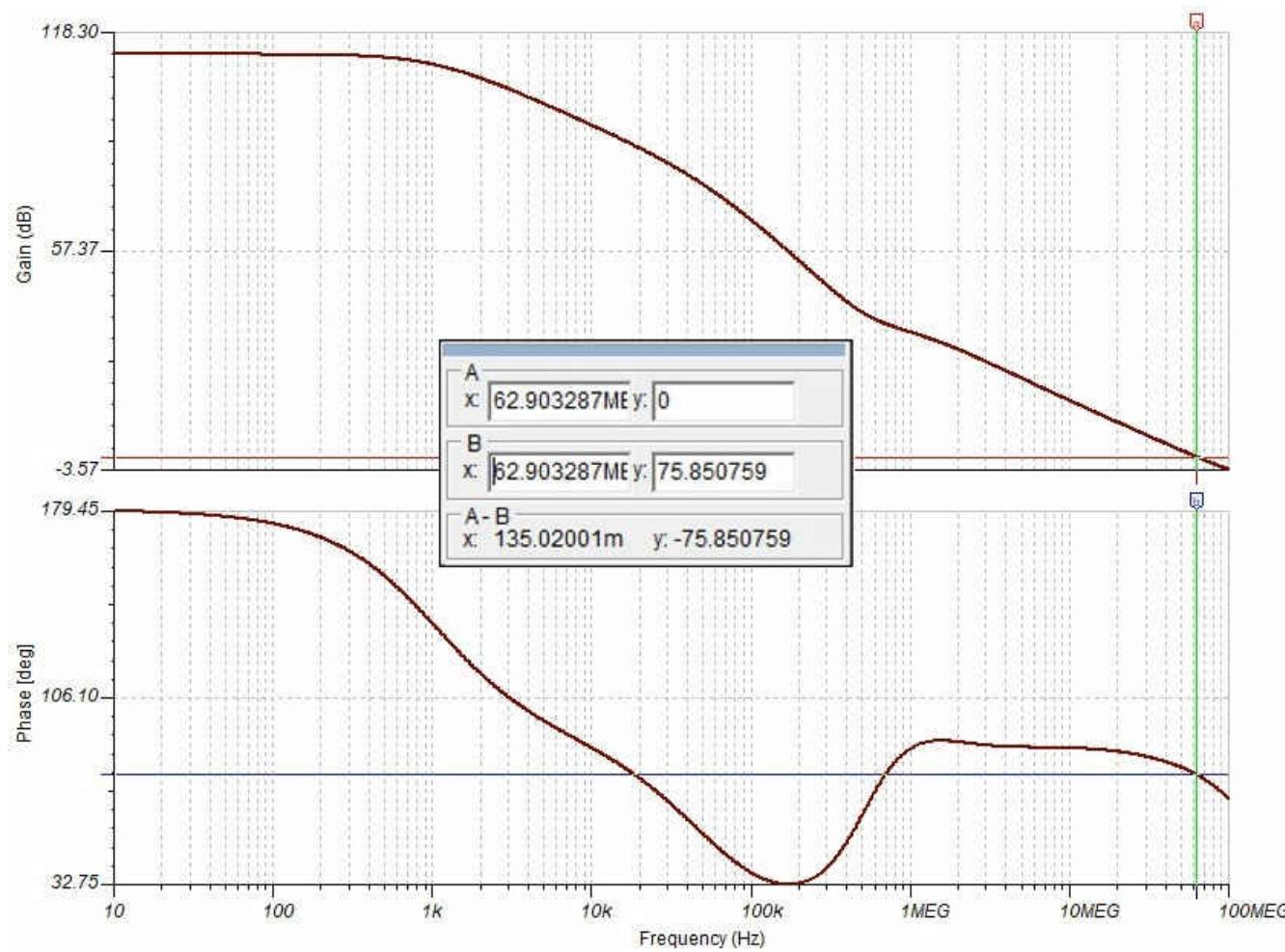
**Figure 2-12. Bode Plot for the FDA Stage in Open Loop Configuration**
