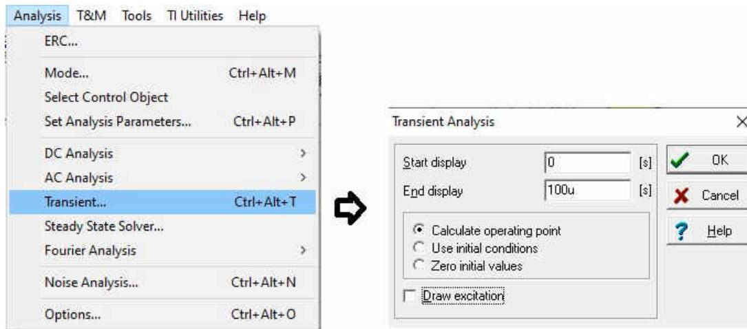
**Figure 2-2. Running the Transient Analysis From 0 to 100  $\mu\text{s}$**
