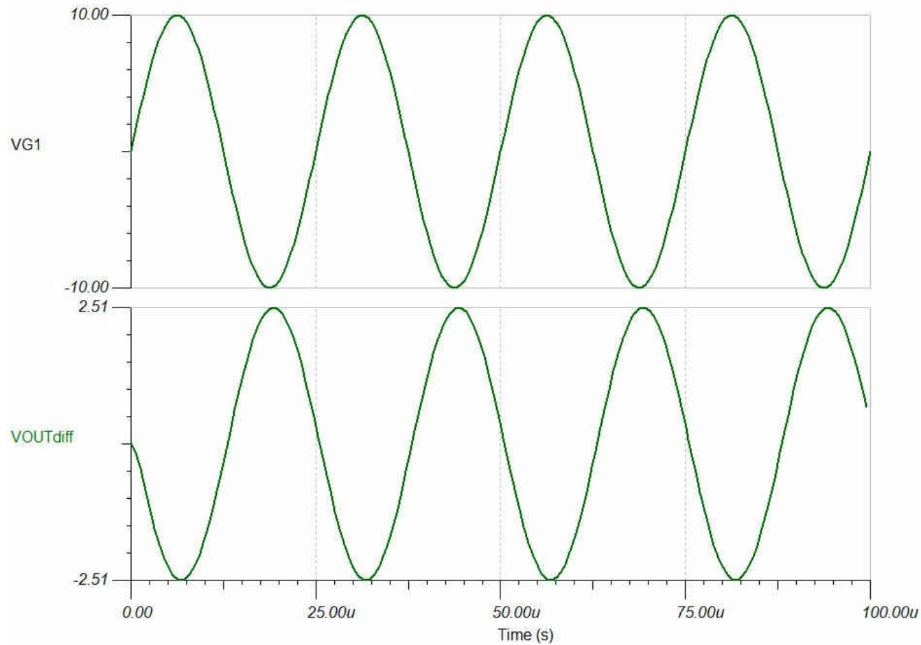
**Figure 2-3. Simulation of FDA Output Voltage VOUTdiff Versus Input Signal VG1**
