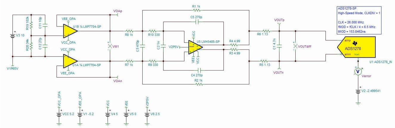
**Figure 2-14. Complete AFE System for Settling Time Analysis**
