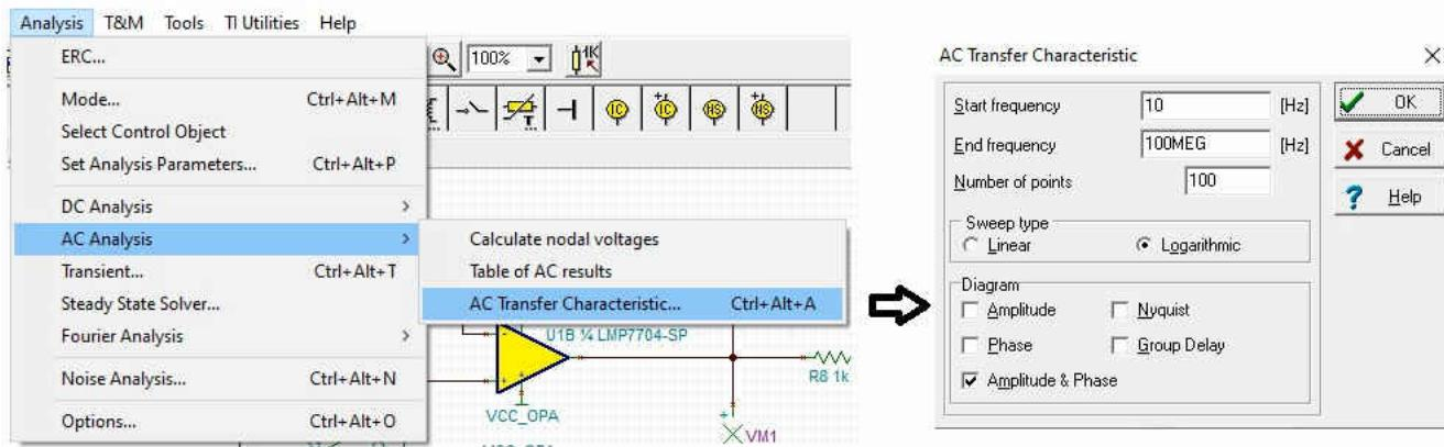
**Figure 2-8. Select AC Transfer Characteristic to Analyze the Frequency Response of the Input Circuit**
