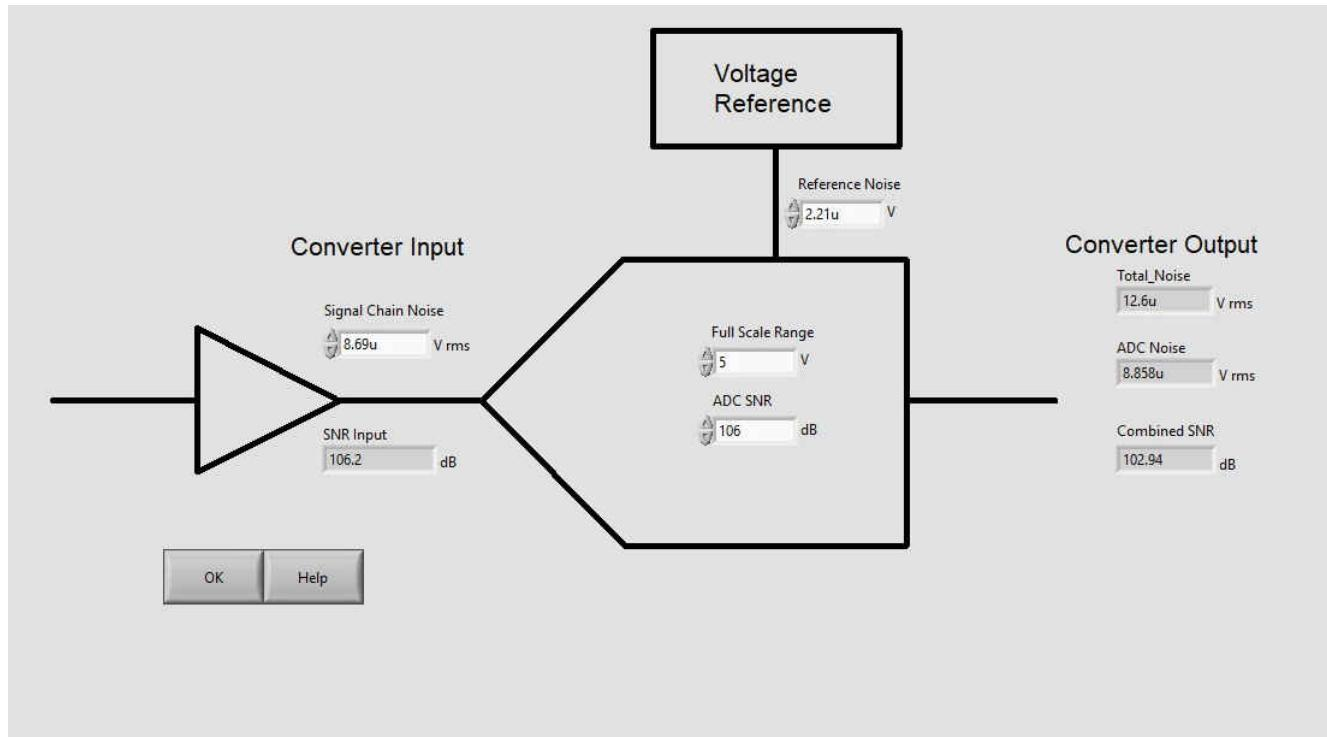
**Figure 2-4. 'ADC + Signal Chain Noise' Analysis in ANALOG-ENGINEER'S CALCULATOR**
