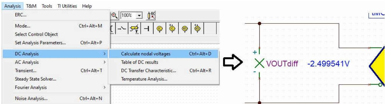
**Figure 2-13. Use DC Analysis → Calculate Nodal Voltages Option to Identify the Precise Input Voltage to the ADC**
