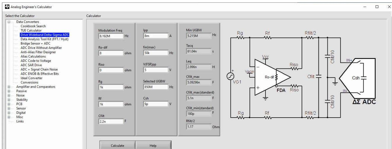
**Figure 1-2. ANALOG-ENGINEER'S CALCULATOR – Drive Wideband Delta-Sigma ADC**
