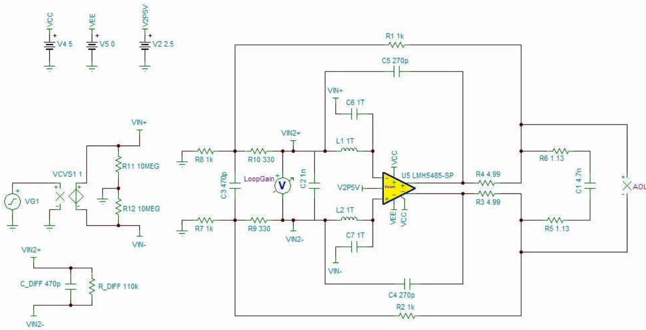
**Figure 2-10. Closed-Loop System Extracted and Prepared for Stability Analysis**
