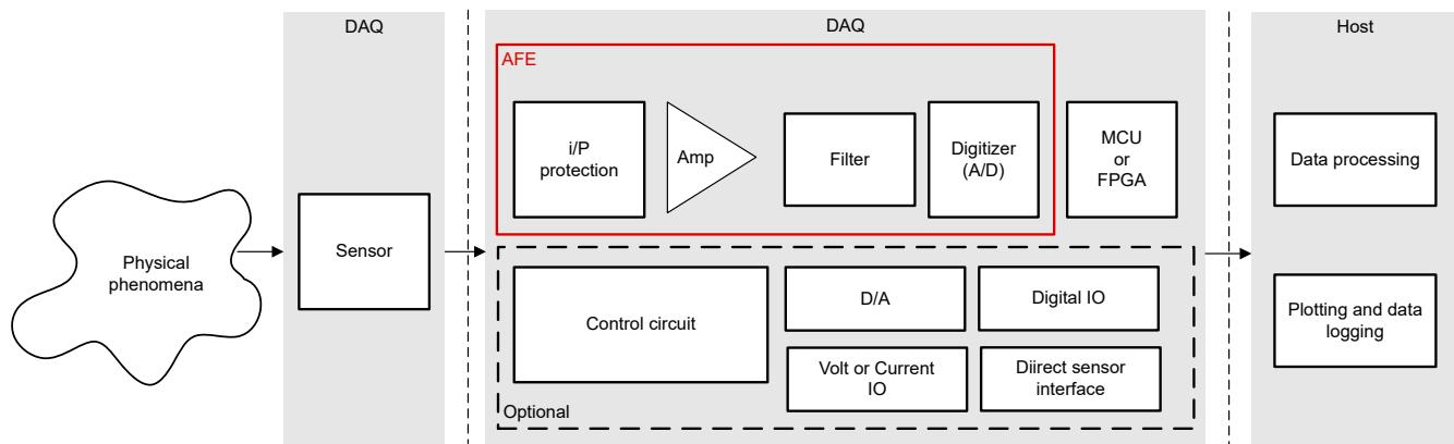
**Figure 1-1. Analog Front-End in a Typical Data Acquisition System**
