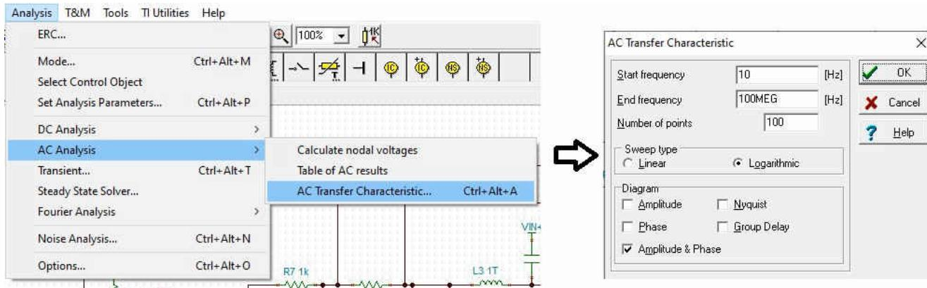
**Figure 2-11. Selection of AC Transfer Characteristic to Analyze the Frequency Response for Amplitude and Phase for the FDA Stage in Open Loop Configuration**
