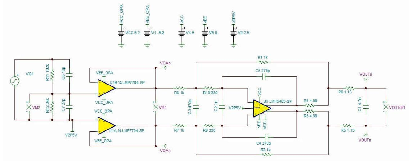
**Figure 2-1. Addition of Attenuation Stage and Input Buffer Stage to the FDA Circuit**
