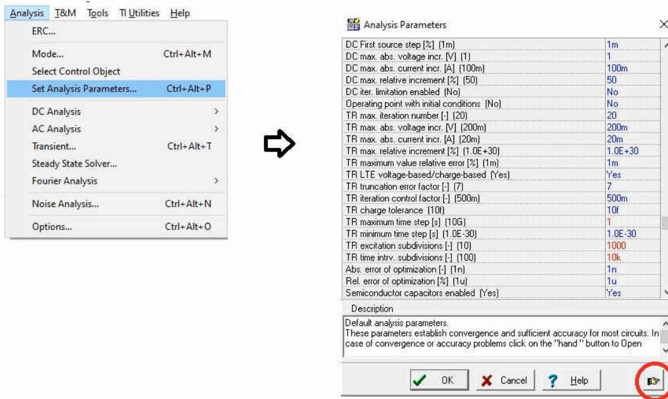
**Figure 2-17. Adjusting Analysis Parameters for High Resolution (Numbers in Red), Press On the ‘Hand Icon’ to Get the Full List**
