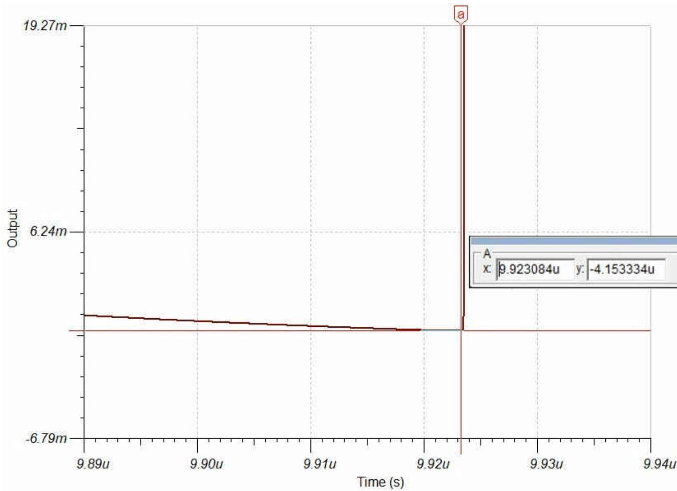
**Figure 2-16. Simulation Result of the Sample-and-Hold Capacitor Voltage Error of the ADS1278 at the End of the Settling Window**
