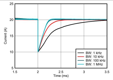
Figure 3-3. DC/DC Step Load Response vs Current Sensor Bandwidth
