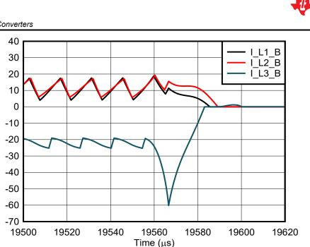
Figure 2-12. Zoomed-in Portion at t = 19.5ms (Span 120µs): Short-Circuit Response of the AC/DC Converter
