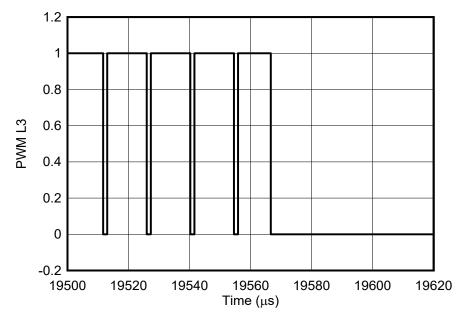
Figure 2-13. Zoomed-in Portion of PWM at t = 19.5ms (Span 120µs): PWM Turn-off Behavior
