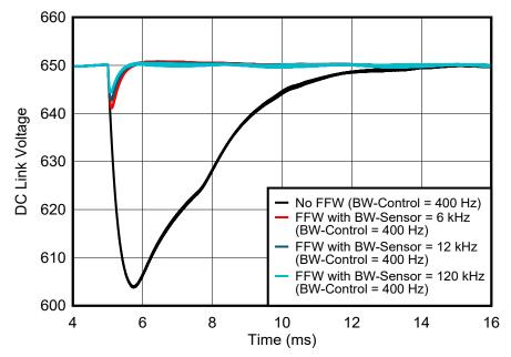
Figure 2-17. DC-Link Voltage Response to Step Power With DC-Link Bandwidth as Parameter, With and Without Feedforward
