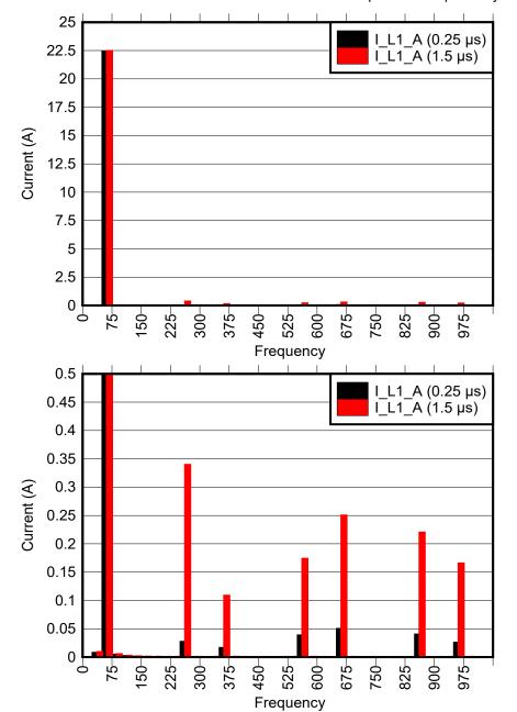
Figure 2-7 shows the results of FFTs of the currents in the PCC when full power is required by the grid.
