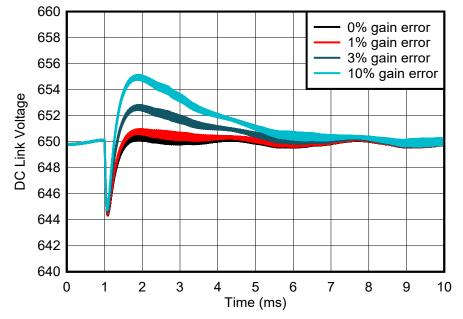
Figure 2-19. DC-Link Voltage Response to Step Power With DC-Link Gain Error as Parameter, With Feedforward
