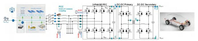
Figure 1-1. Current Sensing Points of an EV Charging System
