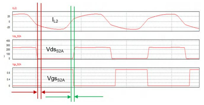
Figure 3-7. Propagation Delay of Zero Crossing Detection
