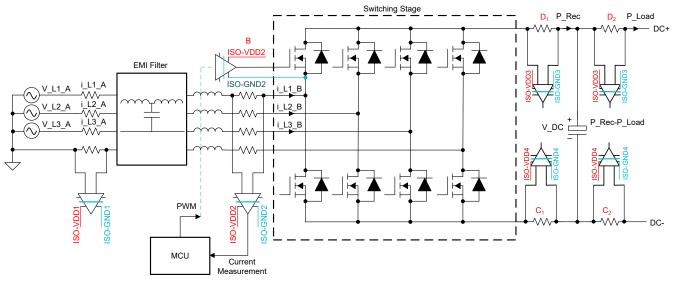
Figure 2-1. Schematic Representation of a Two-Level AC/DC Converter
