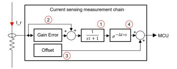
Figure 1-2. Current Sensing Measurement Model
