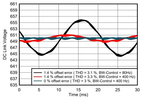
Figure 2-16. DC-Link Voltage Ripple Over Time With DC Link Bandwidth and Offset Error as Parameters
