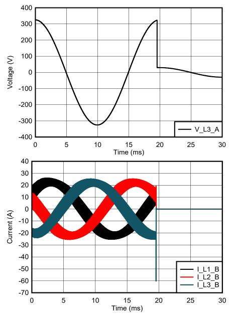
Figure 2-11. Grid Voltages and Currents of AC/DC Converter: Short-Circuit Response of the AC/DC Converter
