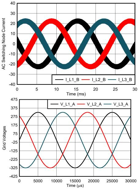
Figure 2-4. Grid Voltages and Currents of an AC/DC Converter Working at the Nominal Load of 11 kW
