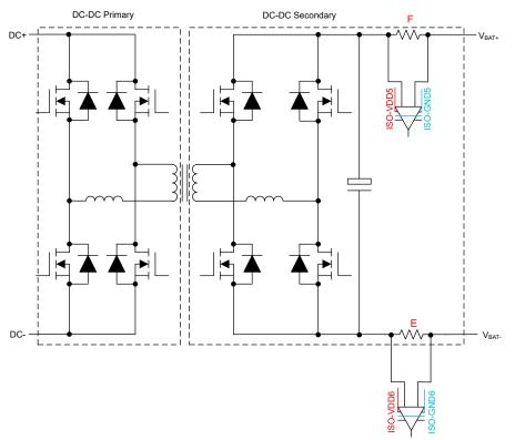
Figure 3-2. Current-Sensing Point E, F
