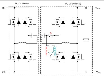
Figure 3-6. Current Sensing at Primary or Secondary Tank of Isolated DC/ DC Converter
