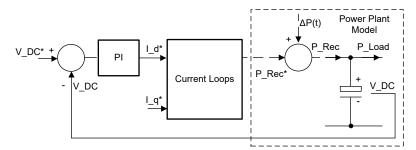
Figure 2-14. Simplified DC Bus Voltage Control Loop With Power Plant Model
