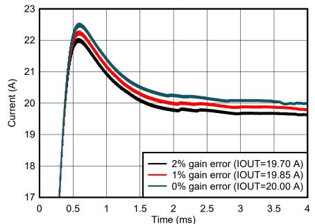
Figure 3-4. Steady State Output Current Errors vs Current Sensor Gain Errors
