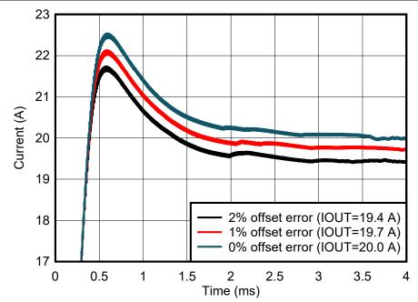
Figure 3-5. Steady State Output Current Errors vs Current Sensor Offset Errors
