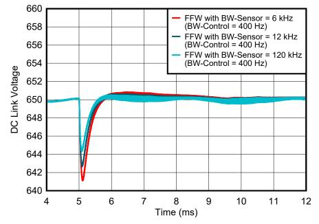
Figure 2-18. DC-Link Voltage Response to Step Power With DC-Link Bandwidth as Parameter, With Feedforward
