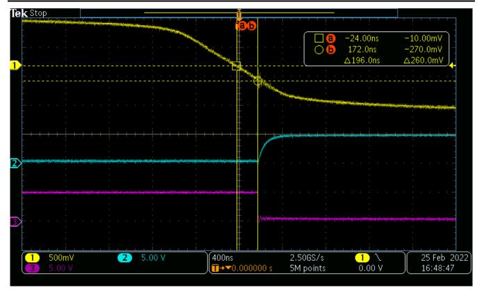
Zero-Crossing Detection Output Latency – Falling Edge
