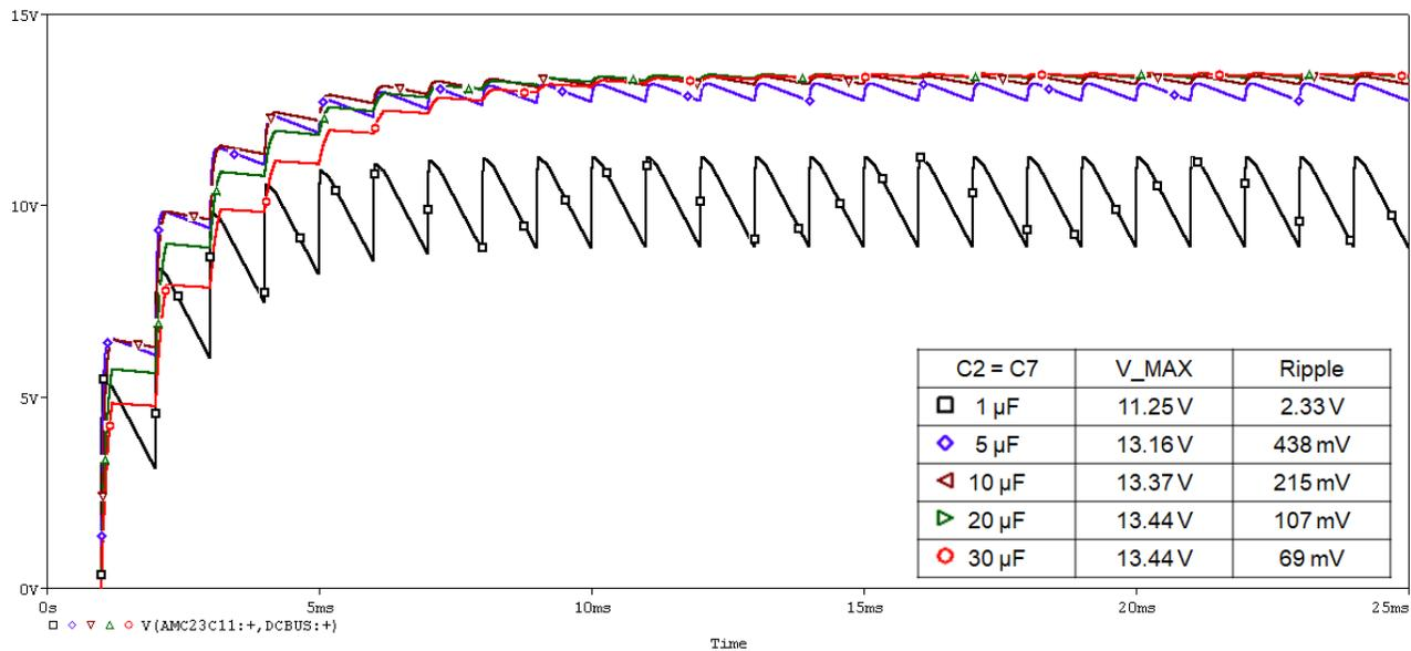
**Figure 3-4. Increase Capacitor Value From 1  $\mu\text{F}$  to 30  $\mu\text{F}$**
