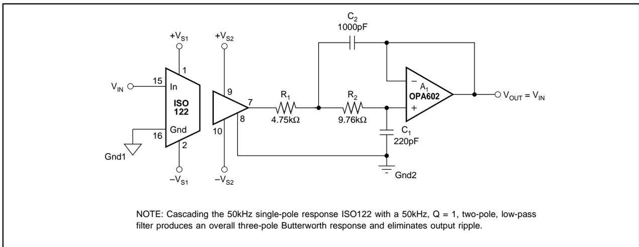
FIGURE 1. ISO122 with Output Filter for Improved Ripple.
